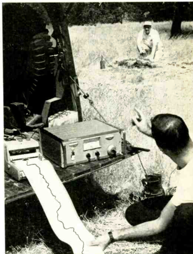
Fig. 6. External magnetic fields cause a change of 4.67 Hz per gamma in the absorption frequency of the rubidium vapor. The oscillator's flicker frequency, once begun, is self-sustaining throughout.
