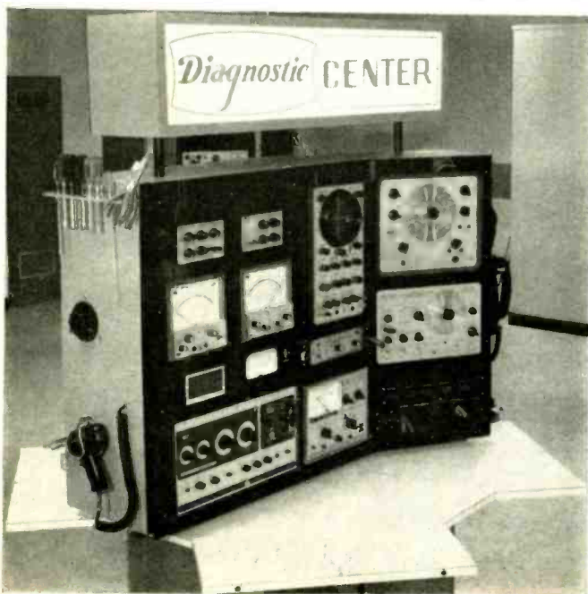
← Fig. 1. Bench and equipment used by the coordinating technician at one of the troubleshooting islands. In addition to the tools, phone, variable autotransformer for line-voltage adjustment, and special test panel at the lower right, the following pieces of test equipment are installed: resistor decade, capacitor decade, transistor tester, v.t.v.m., monitor speaker, line-voltage meter, TV analyst, oscilloscope, color-bar generator, CRT tester, marker and sweep generators.
