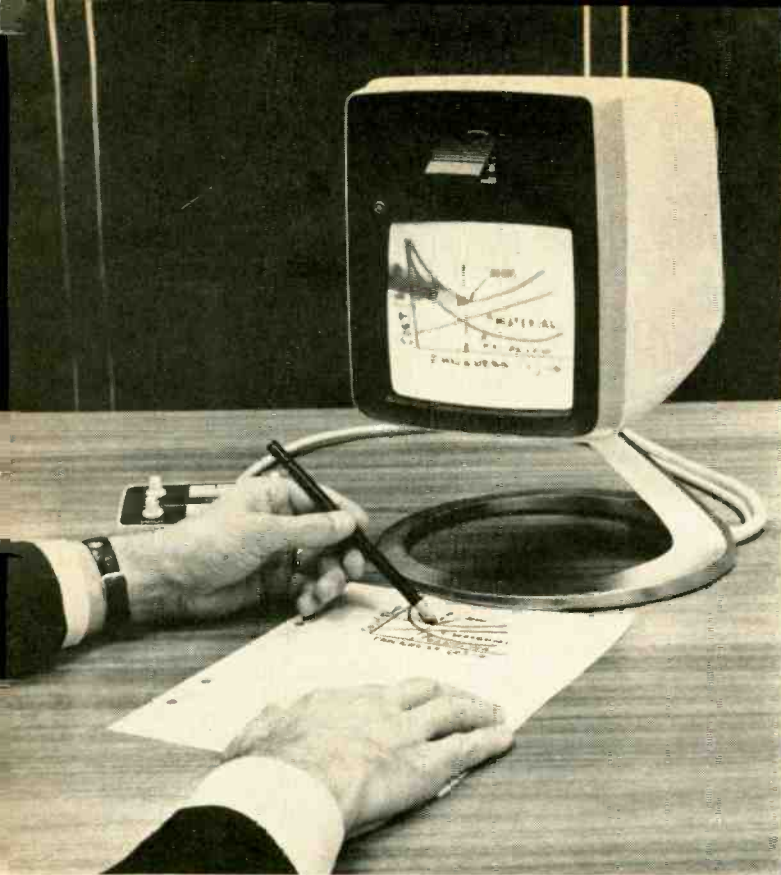
The new Picturephone can transmit drawings or charts which are placed on the desk before it. The "self-view" feature is being used so that the operator can locate his chart properly and see what he is transmitting. Note the small mirror above the lens opening to reflect image into lens.
