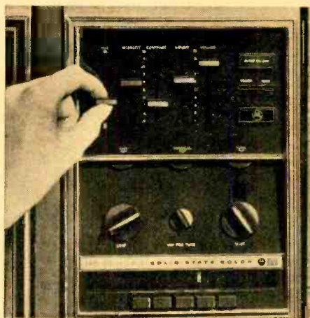
Front panel of new Motorola solid-state set. Slider-type controls are a major feature, but push-button u.h.f. tuning is something new, too. The latter wouldn't be possible without automatic frequency control in transistorized u.h.f. tuner.
