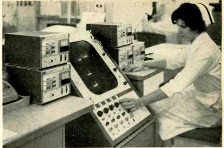
Intensive-care monitoring unit permits continuous monitoring of patients' blood pressure, respiration, electrocardiograms, and electroencephalograms.
