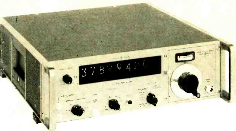
Electronic counter having a 300 to 3000 MHz plug-in unit.
