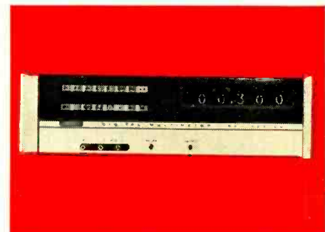
The Cohu Electronics 530 Series digital voltmeter can be used to measure d.c. voltage from 10 mV to 1 kV (actually 999.99 V) with an accuracy of 0.005% of reading \pm 1 digit and d.c./d.c. ratios up to 99.999 to 1. Additional functions, including d.c. current, resistance, and a.c. voltage, can also be provided at additional cost. The price is $1495.
