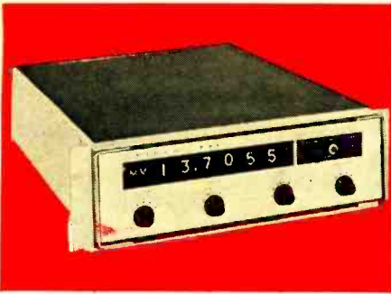
The Vidar 520 is an integrating digital voltmeter that also provides frequency counting, period measurements, and voltage-to-frequency conversion. Its range for voltage measurement is from 10 mV to 1000 V full-scale. The accuracy is \pm 0.01\% of full-scale, \pm 0.004\% of reading. Price is $3925.
