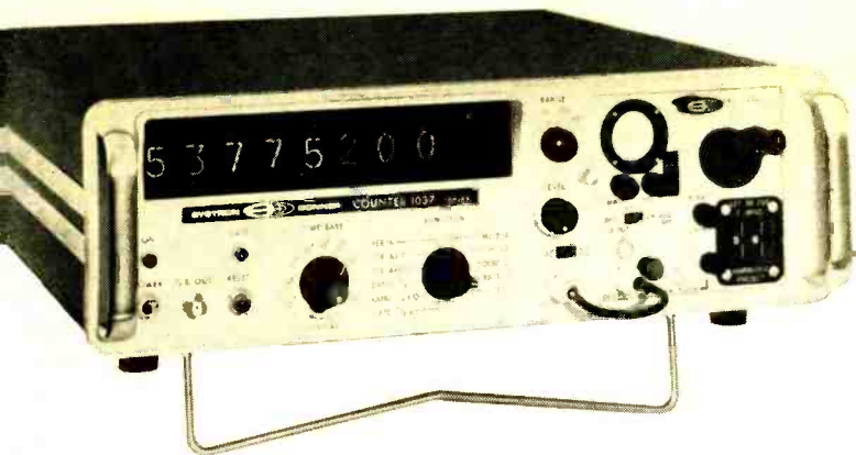
Laboratory counter using a 15,000-MHz transfer oscillator plug-in unit. Other plug-ins cover different frequencies.
