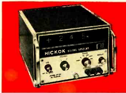
The Hickok DMS-3200 is a digital measuring system. It can be used to measure a variety of electrical parameters depending on the plug-in unit used. As a voltmeter, it measures up to 999 volts with a 0.1% accuracy. Other plug-ins convert unit to counter, ohmmeter, capacitor meter. Main frame: $320.
