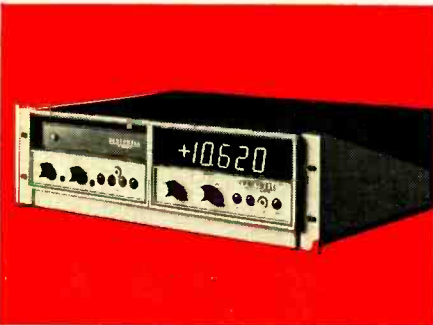
Honeywell Model 620 guarded, differential-input d.v.m. measures d.c. voltages up to 750 V and d.c./d.c. ratios in the presence of high noise levels. Accuracy is \pm 0.01\% of reading or of full-scale. Accessory unit at left is Model 623 converter which adds a.c., resistance, and low-level d.c. measurements. Price of the system begins at $2080.
