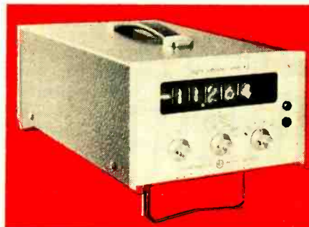
Non-Linear Systems Model X-2 is a small-size integrating d.v.m. with multimeter capabilities. A.c., resistance, and low-level d.c. measurements can be obtained by plugging in appropriate circuit boards. Full-scale d.c. ranges are up to 999.9 V with a rated accuracy of \pm 0.01\% of full-scale and \pm 0.05\% of the reading, \pm 1 digit. Price: $980.
