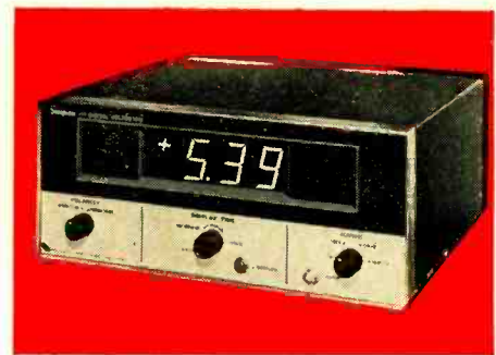
Simpson Model 111 measures from 0 to 999 volts in four ranges. Display time is variable from 200 ms to 10 s. Accuracy is 0.1% of reading, \pm 1 count. The readout is by means of a seven-bar numerical display that can be read out to about 20 feet even under high ambient lighting. Price of unit $500.
