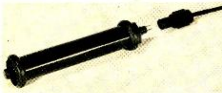
Fig. 9. The oceanographic quartz thermometer probe contains an AT-cut crystal, LC-cut crystal, reference oscillator, temperature oscillator, and mixer. The pressure case at left withstands 10,000 psi.
