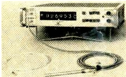
Fig. 8. The probes of this quartz thermometer each contain an LC-cut type crystal. They are connected by coaxial cable to the electronic chassis. The cables carry 28-MHz signals. (Dymec Div., Hewlett-Packard)
