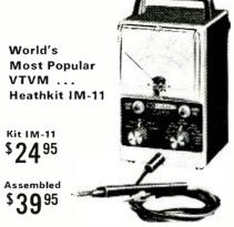
• 7 AC, 7 DC, & ohms ranges — easy-toread scales • 4½", 200 uA meter • 1% precision resistors for high accuracy • Extended frequency response,  $\pm$ 1 db 25 Hz to 1 MHz • Measures RMS and Peak-to-Peak • Single test probe for all measurements • Easy-to-build, electronically stable circuit board construction • Costs just 45c more than its predecessor of 16 years ago. 5 lbs.
