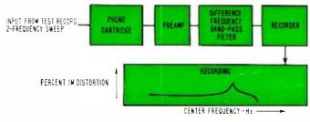
Fig. 6. Setup used for making the CCIF distortion measurement.
