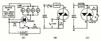
Fig. 4. (A) Basic application of SCR in a lamp-driver circuit. (B) Basic application of a gated bi-directional controlled rectifier. (C) The power line triggers the gated bi-directional controlled rectifier when switch S1 closes.
