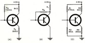
increased input impedance, the emitter resistor may be bypassed with a capacitor, while maintaining the d.c. bias stability. One means of maintaining a constant d.c. bias stability is to heat-sink the transistor, although this is usually not feasible for small transistors. Another method is to use stabilizing components to avoid runaway.
