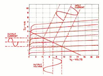
Fig. 3. Use of load line to show input and output currents, voltage.
