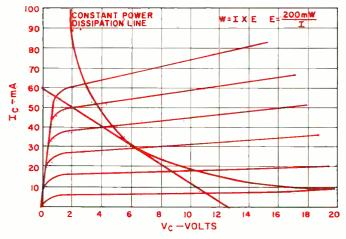
nal would be shown as a clipped, negative-going output voltage waveform, since the transistor would be saturated at this point. This would indicate that either the load resistor is too high (reducing collector voltage) or the bias resistor is too low (increasing base current).
