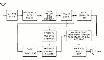
Fig. 1. When the RRA system picks up a tone-coded CB signal, a prerecorded tape takes over the car radio. Should a prior:ty signal come in, it overrides other signals.
