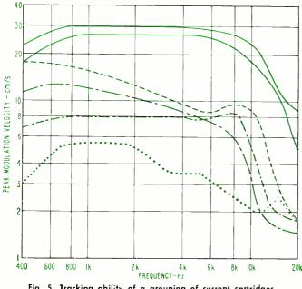
Fig. 5. Tracking ability of a grouping of current cartridges.
