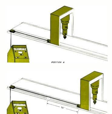
Fig. 3. An example of using a laser interferometer. Position A is the starting or zero point. At position B, the table has been moved 50 inches. Readout is by counter.
