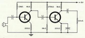
below a one-volt level. This represents a voltage ratio of 500; hence the preamplifier should have a voltage gain of 500 from input to output to drive a power amplifier with one volt r.m.s.
