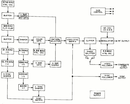
the receiver. The "Color Gun" control provides a means of making fast purity checks without disturbing the color screen controls of the receiver. Use of the gun control will also allow individual R-Y, B-Y, and G-Y displays to be viewed, thereby utilizing the picture tube to check color demodulation outputs and eliminating the need for an oscilloscope.
