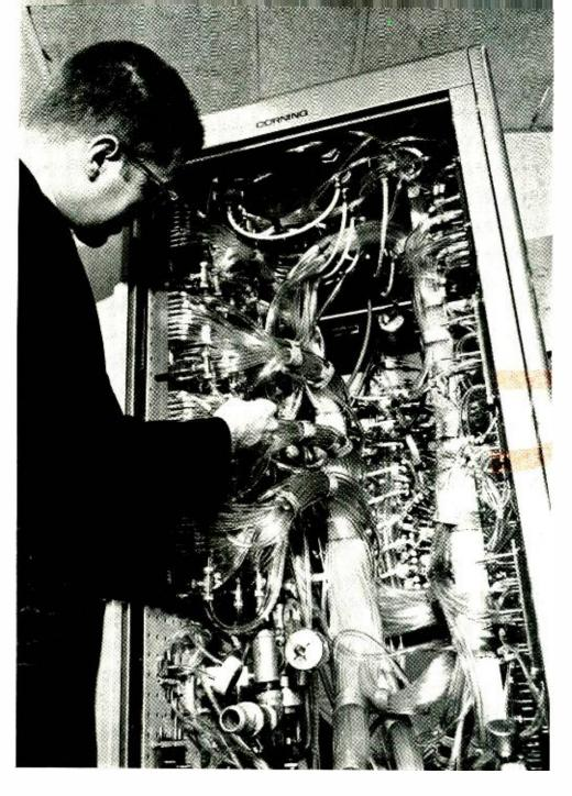
A fluidic time-based sequencer used to control a glass press is shown here. This digital control system, the most complicated fluidic system ever assembled, contains 1050 standard active and passive devices in a relay rack two feet square by six feet high. It will replace an electromechanical press control that requires manual adjustment of valve-actuating cams taking more than an hour for setup. Fluidic control setup time is under 15 min.
