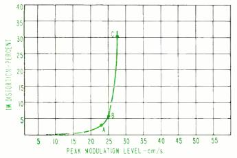
Fig. 1. Intermodulation distortion for various peak modulation levels (actually recorded velocities) for phono cartridge tracking at 1 gram. Frequencies are 400 and 4000 Hz on RCA 12-5-39 test record. Although level is fairly high at point A, distortion is still acceptably low. At point B distortion begins to rise rapidly ultimately reaching excessively high value at C.
