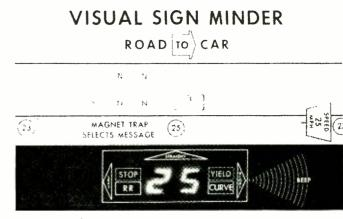
Fig. 6. In the DAIR system, passing over magnetic traps produces a driver alert tone and indicates the message.
