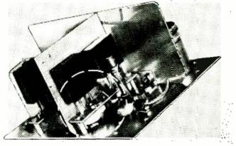
Fig. 5. Method of mounting crystals on the crystal trimmers.
