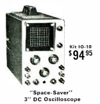
• Identical vertical & horizontal DC or AC coupled amplifiers • DC to 200 kHz bandwidth - less than 5° phase shift • Recurrent sweep generator, 5 Hz to 50 kHz in four ranges • External capacitor binding posts for slower sweep rates . Small, compact, easy to carry from job to job • All critical voltages regulated for high stability Transformer operated power supply. 16 lbs.
