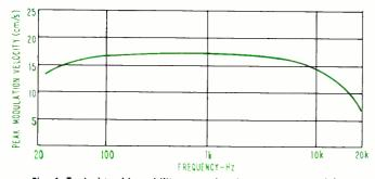
Fig. 4. Typical tracking-ability curve showing maximum modulation velocity the cartridge can track as function of frequency.
