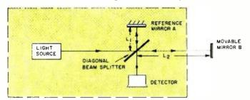
Fig. 1. Operation of the basic Michelson interferometer.
