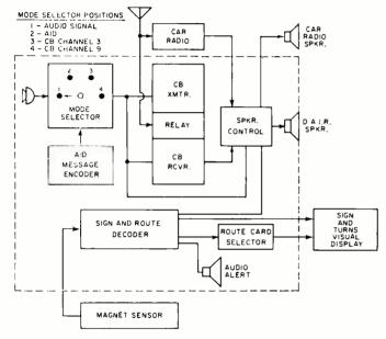
Fig. 4. The DAIR system uses either CB or signals from buried permanent magnets to activate the readout systems.
