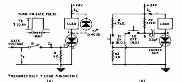
Fig. 2. (A) Basic SCR latching circuit. (B) An SCR latching circuit using a commutating capacitor to assist operation.
