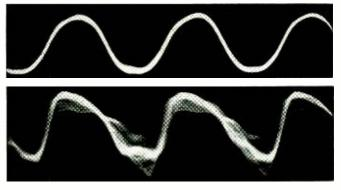
Fig. 2. Upper waveform is from a cartridge that is just barely tracking the sine-wave modulation. Lower waveform shows distortion produced when cartridge is not tracking.
