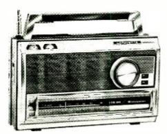
medium-wave bands while a multi-section whip is provided for short-wave and FM reception. The two-way speaker system consists of a 4" woofer and a  $1\frac{1}{2}$ " tweeter. There are separate jacks for external antenna, earphone, a.c. (with optional adapter), speaker, and phono. The unit measures  $13'' \times 8'' \times 5''$  and requires six "C" cells for operation. Lafayette
