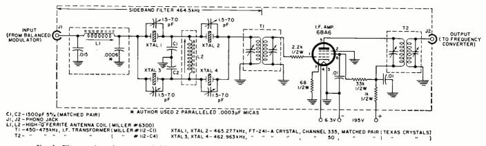
Fig. 1. Filter consists of two cascaded half-lattice crystal-filter sections with low-impedance input and high-impedance output.
