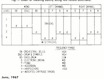
Fig. 7. Chart of tracking ability using test record described.
