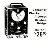
• Tests all capacitor types • Low bridge voltage for safe testing of miniature electrolytics • 16 leakage testing voltages = Direct reading scales — no involved calculations • Measures resistance from 5 ohms to 50 megohms • Measures caparator circuit — measures "L", "C", or "R" with external standard • "Eye" tube null & leakage indicator. 7 lbs.
