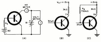
Fig. 2. (A) Setup for obtaining characteristic curves. (B) Operation with 3000-ohm load and (C) with a 6000-ohm load.
