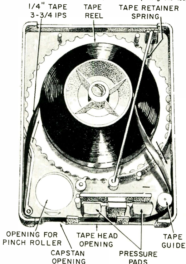
Fig. 1. The Fidelipac ( TelePro ) cartridge consists of a single reel of specially lubricated tape arranged as a continuous loop. The tape comes off the center of the reel and moves around the tape guide and past the two pressure pads and tape head. It then goes between pinch roller and capstan which are on the tape deck and engage the tape through openings in cartridge. The tape then returns to the outside of the tape reel, completing the loop.
