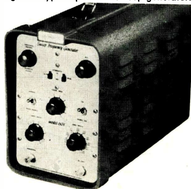
Fig. 13. Typical portable sweep generator.
