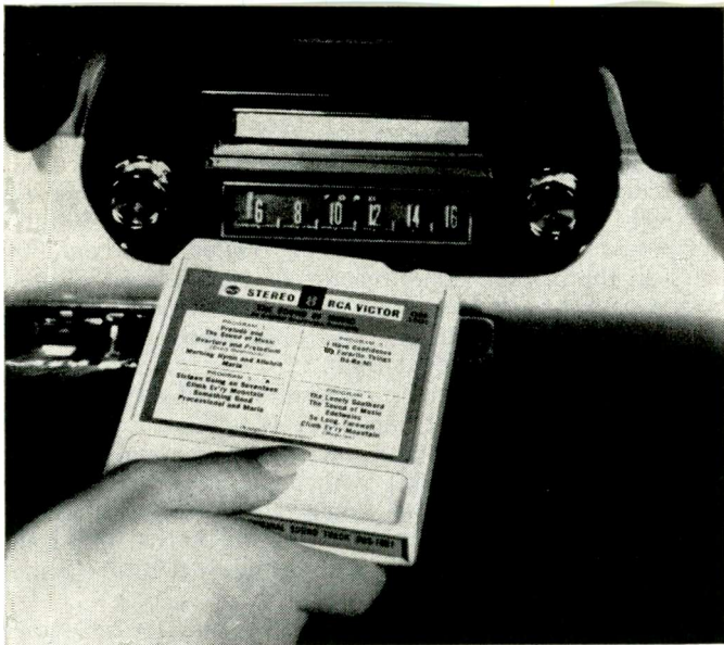
Lear cartridge is about to be inserted into opening above dial of this combination automobile radio and tape playback unit.
