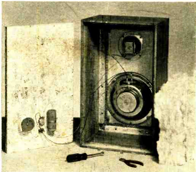
After the fiberglass is put in the cabinet, back is screwed on.
