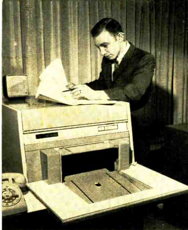
Preparing to tune up a long-distance xerography scanner, Levit traces a supervisory signal through the computer logic schematic.
