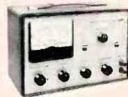
New Model 378 Audio Generator. Near-distortionless sine wave generator (<0.1% 20-20,000c) providing fast, convenient switch-selection of frequencies from 1c to 110kc (1c steps 1c-100c, 10c steps 100c-1kc, 100c steps 1kc-10kc, 1kc steps 10kc-110kc), 8-pos. 10db/step output attenuator & fine attenuator. Output meter (4 1/2" 200ua) with 8 voltage ranges & db scale. $49.95 kit, $69.95 wired.
