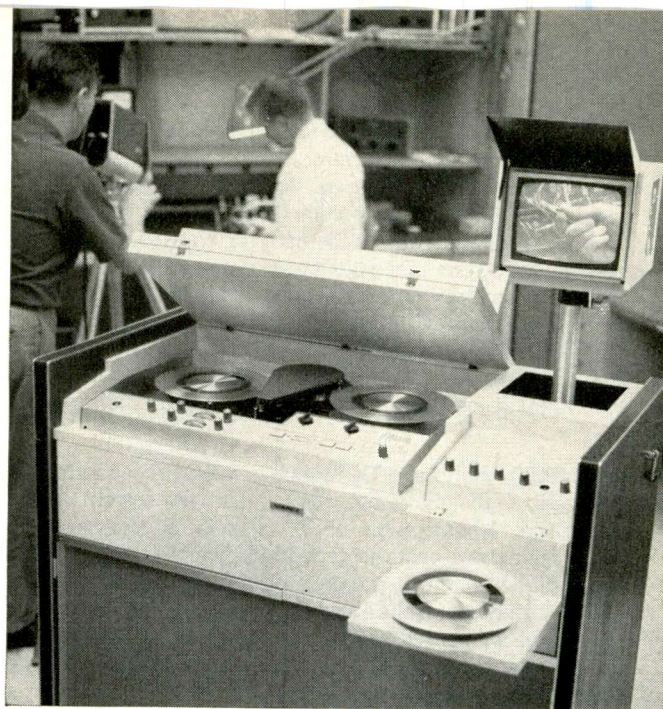
The single-head full-helical video tape recorder may be employed to prepare training tapes for industry or for schools.
