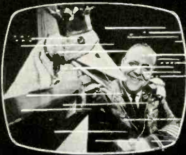
Unshielded twin-lead Severe picture disturbance due to ignition noise.
