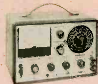
New Model 965 FaradOhm Bridge/Analyzer. "Unusually versatile" — Electronics World. 9-range, low-voltage capacitance-resistance bridge safely measures even 1-volt electrolytics. Metered bridge balance, leakage test voltage (6 DC VTAM ranges 1.5-500V), leakage current (11 DC VTAM ranges 0.15ua-15ma). DC VTVM & VTAM externally usable. $129.95 wired.
