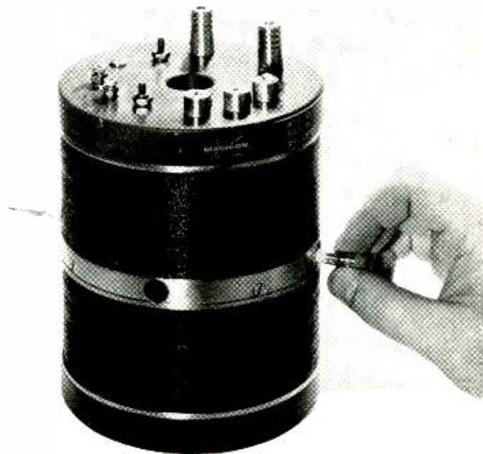
50,000-gauss superconducting magnet used to study properties of matter in high magnetic fields at very low temperatures.
