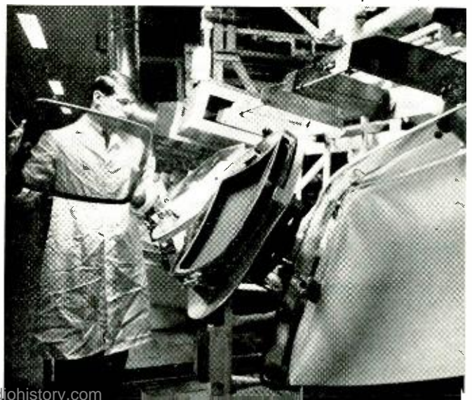
Fig. 7. Installing a shadow mask. The supporting system is so accurate that the mask is oriented within a quarter mil.
