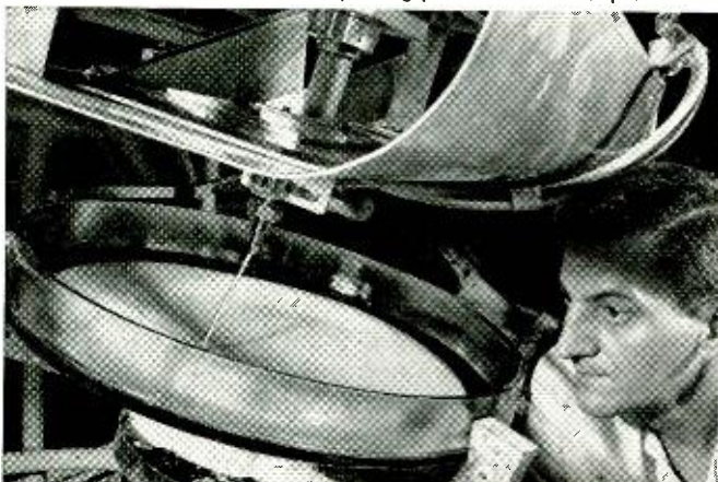
Fig. 6. The phosphor dispensing station deposits an exact amount of phosphor on the spinning panel for uniform spread.
