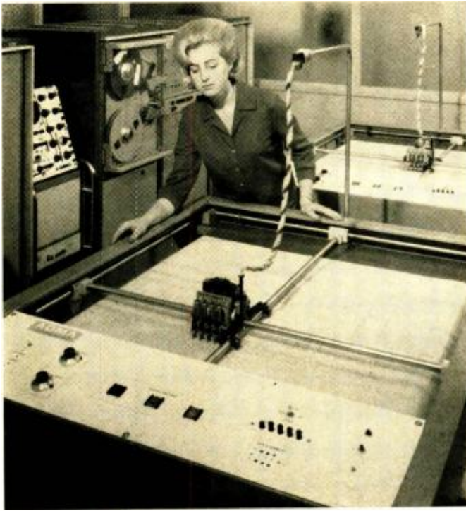
The automatic drafting machine couples a magnetic memory with a servo-controlled x-y plotter to produce sketches.
