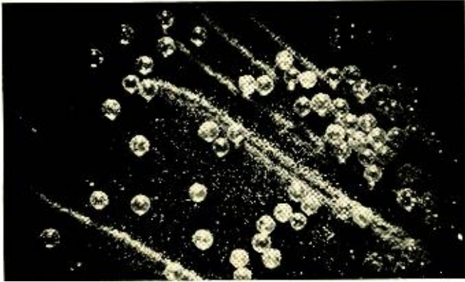
Photomicrograph of xerographic image being formed. The large positively charged carrier beads transport negatively charged toner particles to the positively charged selenium-coated plate. The carrier beads are 100-200 times larger than toner particles. (The dry developer powder is a special formulation of small glass or sand carrier beads plus particles of black heat-fusible carbon.)
