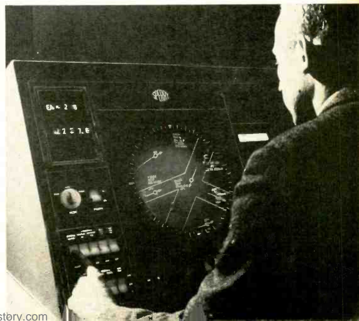
All-Purpose Display Console. (Right) A highly versatile display console has been demonstrated recently that will work with any kind of radar, sonar, or computer. Until now, with the exception of very rudimentary installations, every new radar, sonar, or computer system has required a custom-designed console. The display, which uses plug-in "building-block" components made of microcircuits, tiny wafers that contain entire circuits within their molecular structure, can be used for purposes as different as shipboard sonar and air traffic control radar. Or it can display a line by line message at a rate of over 250,000 characters per second, outpacing most computers. The new all-purpose display console was developed by the Sperry Rand Corp.
