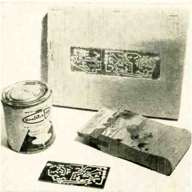
Fig. 6. The finished screen, squeegee, and printed board. Note the use of masking paper around the printed-circuit layout which keeps ink away from borders of layout used.
