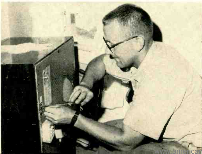
Connecting the cable to a customer's receiver. The impedance-matching transformer is just below technician's left hand.
