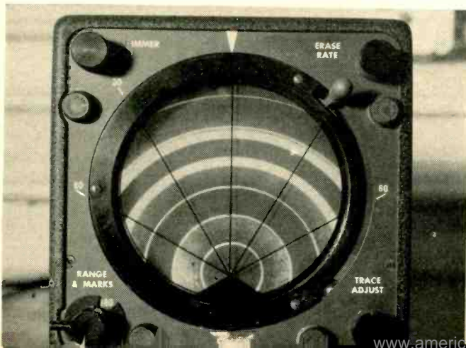
A bright display unit of an airborne weather-radar system. A DVST permits the pilot to view the screen without using a hood. Test pattern shown is used to check radar before taking off.
