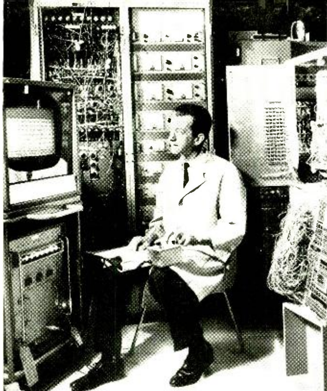
Main units of IBM experimental multifont optical character reader are shown here. Power supply and scanner are in the background, a part of identification circuitry is at right. The text, as seen by the scanner, is displayed on TV screen.
