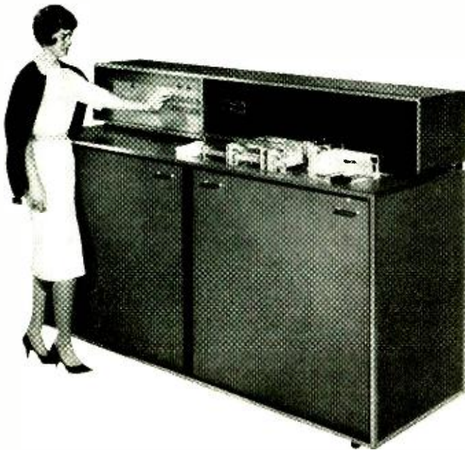
Documents to be read are fed to paper-handling equipment at front of this Farrington reader. Associated electronic equipment, including recognition logic, is housed in the cabinet.
