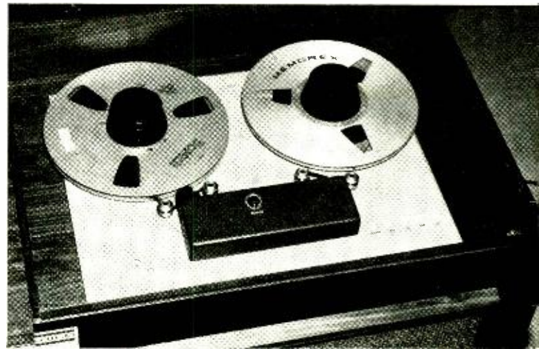
Top panel of the tape transport mechanism. Standard 10½" reels of instrumentation tape were used for the demonstration. The tape has a low-friction high-resolution coating. The "Focus" control emerging from the head cover adjusts the head azimuth. The five push-button controls at right are for record, fast rewind, fast forward (at about 200 ips), playback, and stop. Indicator at left shows which of the four tracks on tape is being recorded or played.
