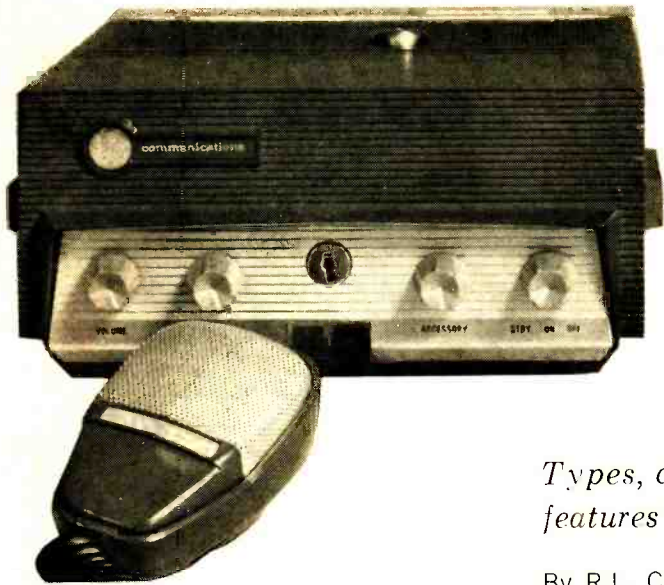
This G-E transistorized mobile communications equipment is furnished with a rugged controlled-reluctance microphone.
