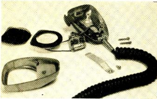
Motorola dynamic mike with built-in transistor amplifier.
