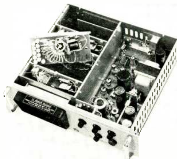
Inside view of the voltmeter discussed. One of the four stepping-switch panels has been unplugged in this photo.
