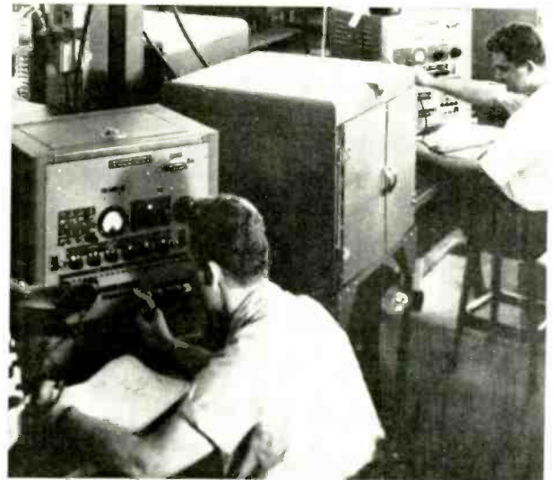
Fig. 4. Subassembly is being subjected to extremes of temperature in the high-temperature test chamber shown in the center.
