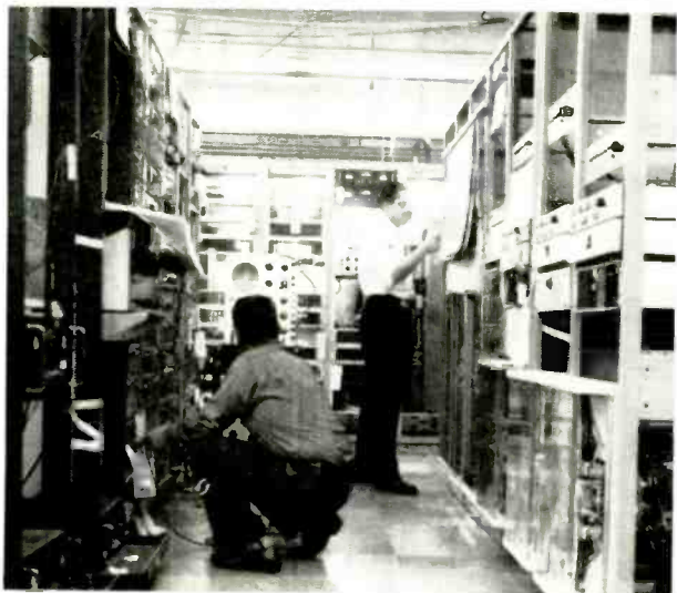
Fig. 5. After breadboard of entire system is completed and assembled, lab technicians perform system tests and debugging.
