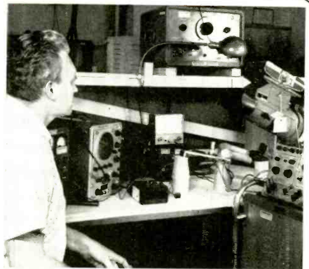
Fig. 2. The operation of a breadboard circuit is checked by a technician using signal generators and an oscilloscope.
