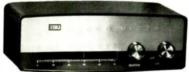
Fig. 3. This top-of-set u.h.f. converter uses a nuvistor in oscillator portion and high-frequency, low-noise transistor as the i.f. amplifier. Output is either v.h.f. Ch. 5 or 6.
