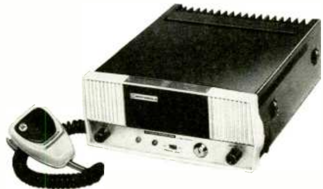
Typical self-contained mobile radio for vehicular mounting.
