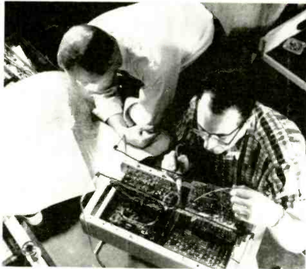
Fig. 1. Lab technician is constructing a breadboard subassembly following schematic prepared under engineering direction.
