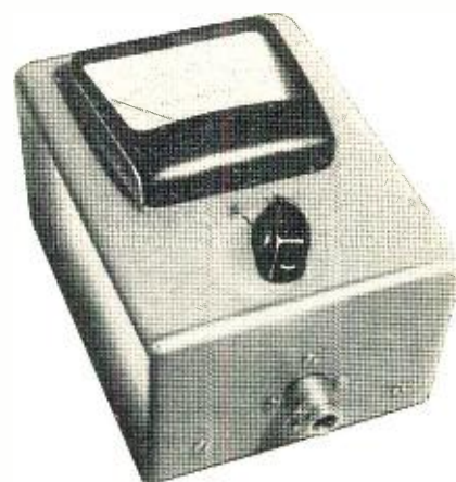
Fig. 4. A typical commercial dual-range r.f. wattmeter unit.
