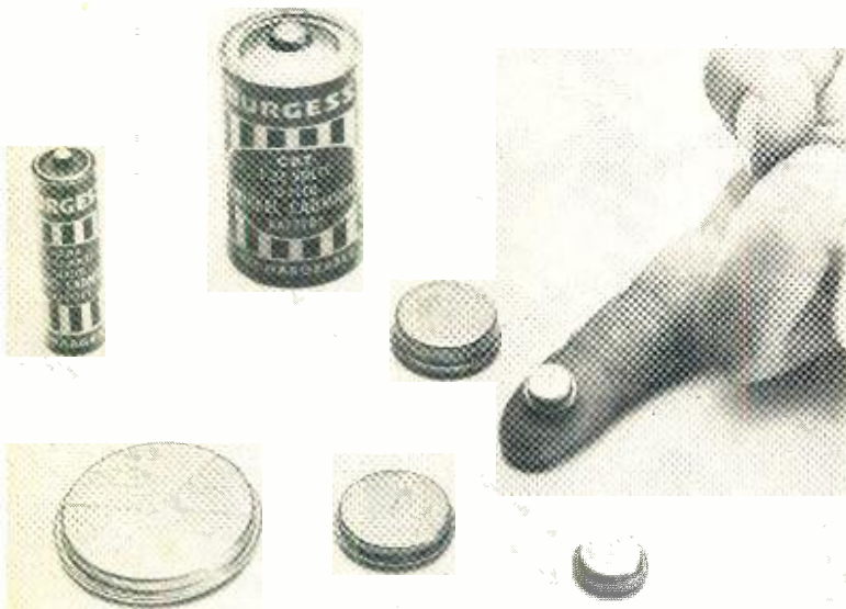
Fig. 5. Various sizes of nickel-cadmium cells can be packaged to make higher battery voltages. The cells are rechargeable.
