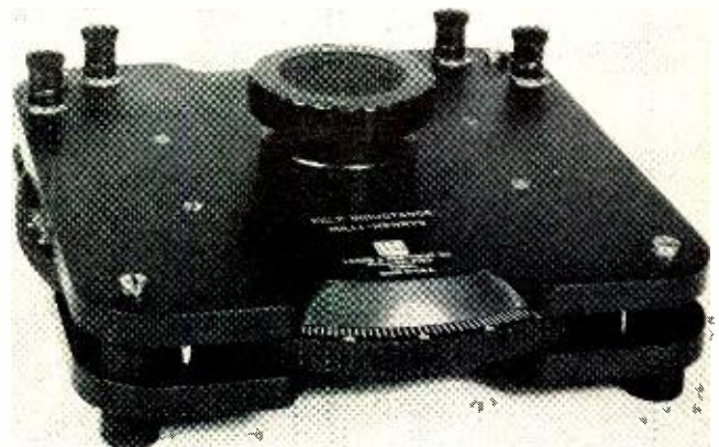
Fig. 7. Three sets of carefully wound coils interact in the Brooks "Inductometer" for inductance readings on a linear scale.
