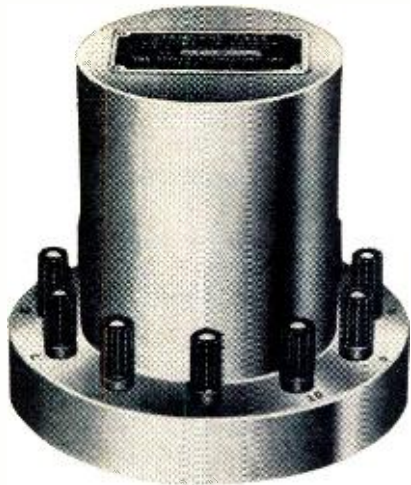
Fig. 1. The Eppley Standard-Cell Voltage Reference, accurate to .005% or better, is tapped in ten steps up to 10.193 volts.
