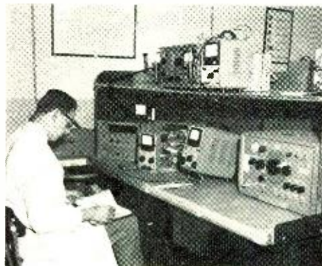
(Left) Technician is shown calibrating a u.h.f. signal generator. (Center) Calibration of a vacuum-tube voltmeter against a standard. (Right) Checking an oscilloscope time base against a master frequency standard.
