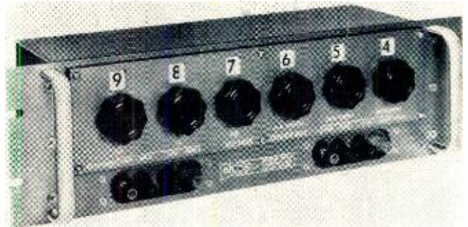
Fig. 4. A resistive voltage divider made by North Hills Electronics. It is made for use with an external voltage source.
