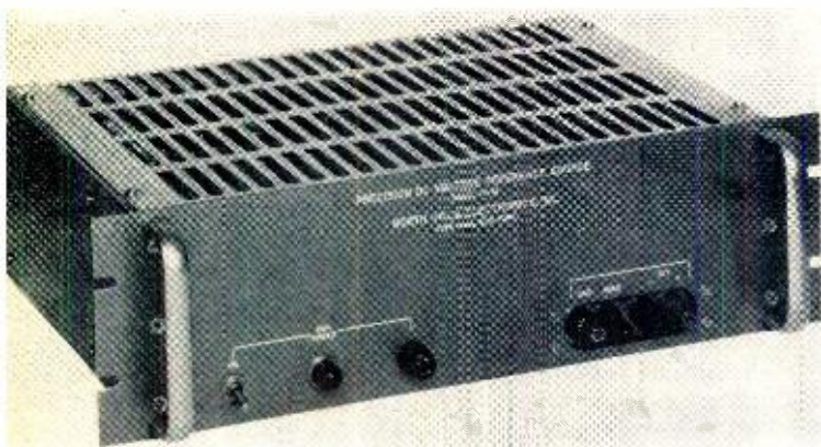
Fig. 2. An a.c.-powered, well-regulated standard, the VS-10 by North Hills Electronics, provides d.c. reference output.
