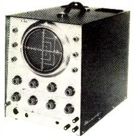
Another example of a general-purpose wide-band instrument designed mainly for black-and-white and color-TV servicing is the Jackson CRO-3. When switched to wide-band operation, the response is from 20 cps to 4.5 mc. When set for high sensitivity, 18 mv. r.m.s. signal produces a deflection of 1 inch. Price of unit is $234.95.
