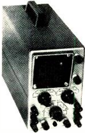
A 3-inch d.c. oscilloscope that is available in kit form is the Heath IO-10. Identical vertical and horizontal channels are used with bandwidths from d.c. to 200 kc. Sensitivities of amplifiers are 0.4 v. (p-p) per inch. This compact scope weighs about 16 lbs. There is less than 5° relative phase shift between channels. Price: $79.95.
