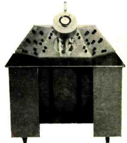
Experimental model of Wilska's short-column low-voltage unit.
