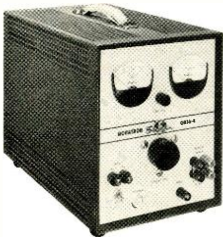
Fig. 3. Portable power supply with output of 0-40 v. at 0-5 amps.
