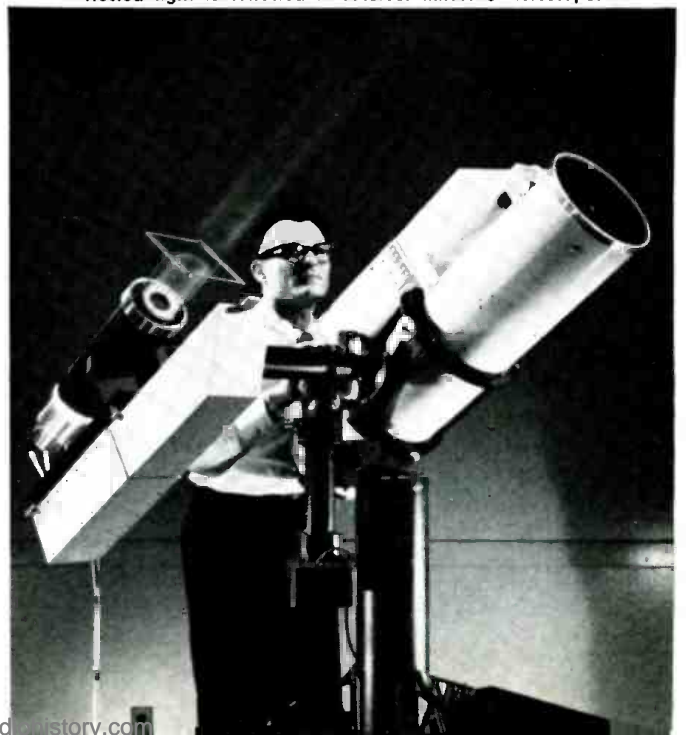
Experimental laser radar devised by Hughes. The laser (at left) produces an intense, tightly focused light beam that is aimed toward a target a number of miles away. The reflected light is collected in receiver mirror of telescope.
