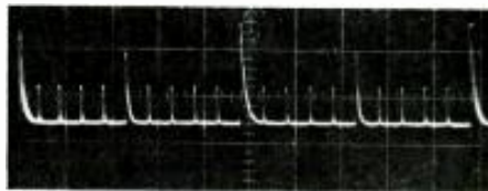
Fig. 3. Train of time-marker pulses displayed with 10 \mu\text{sec./cm.} sweep speed.
