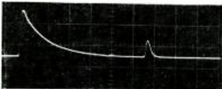
Fig. 5. Intensified portion of waveform fills graticule with 1 \mu\text{sec./cm.} sweep.
