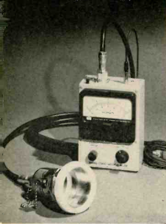
Fig. 1. Electrometer voltmeter equipped with head for measuring static charges.
