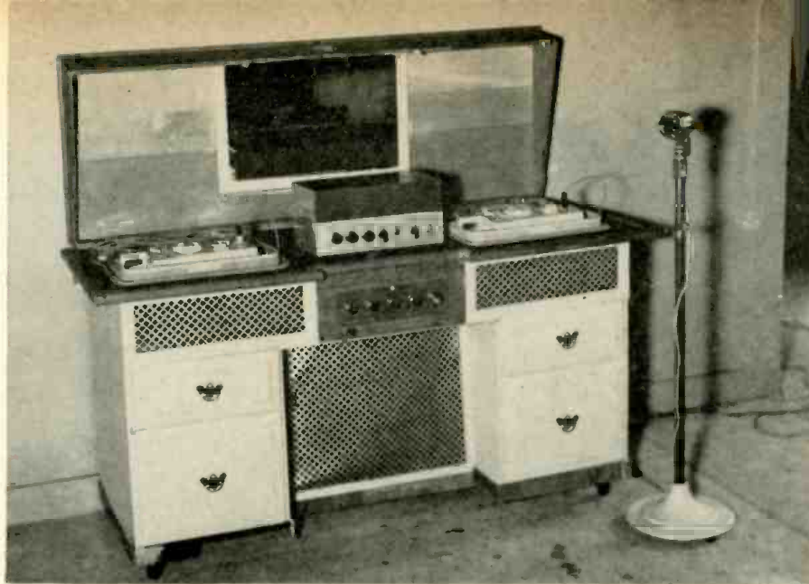
The mixer unit is placed between the two tape recorders. The mirror behind the mixer is used for speech-articulation practice for a near-deaf child.
