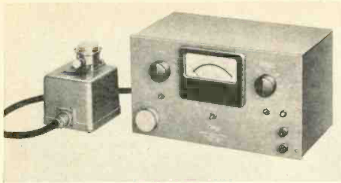
Fig. 5. This vibrating-reed electrometer measures current as low as 10^{-17} amp. Shielded box at left contains preamplifier.
