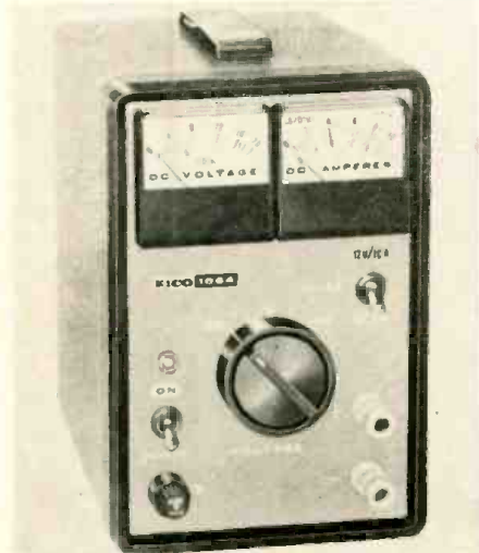
Fig. 1. Float a conventional battery eliminator, like the Eico 1064, across a battery pack for a regulated power source.
