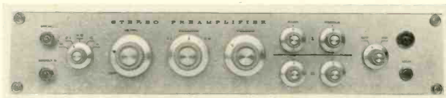
Front panel view of the author's stereo preamp showing the operating controls.
