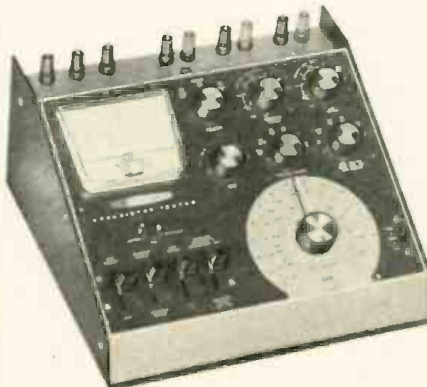
Fig. 12. A supplementary transistor test- er (this one by Heath) is needed if the tube tester lacks this facility. Use of tran- sistors is now common in marine radio.
