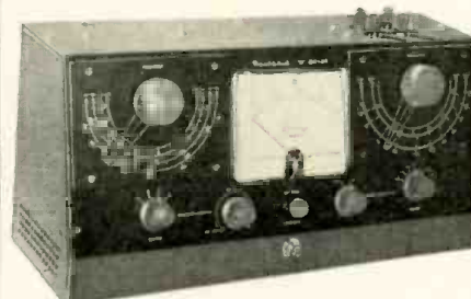
Fig. 10. A "Q" meter, like the Heath QM-1, is useful. High "Q" of antenna-loading coils assures efficiency of transmission.
