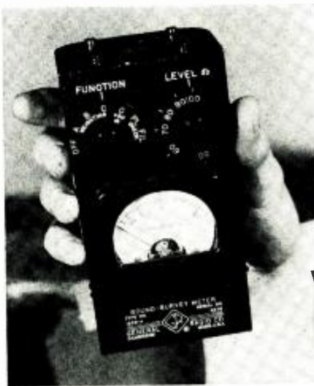
The sound-survey meter is small, easy-to-use, and battery-powered for portability.
