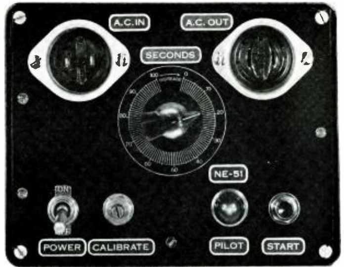
Front-panel view of the linearized thyatron interval timer.
