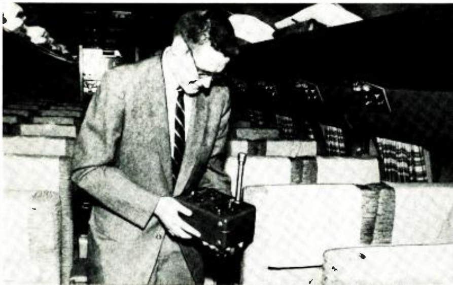
A sound-level meter being used to check the noise level inside an airliner.
