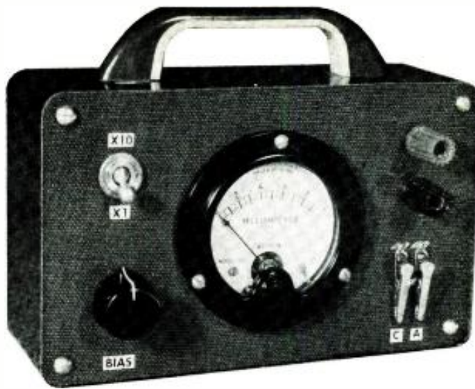
Tester is built into a 6 1/4" x 3 3/4" x 2" Bakelite case.
