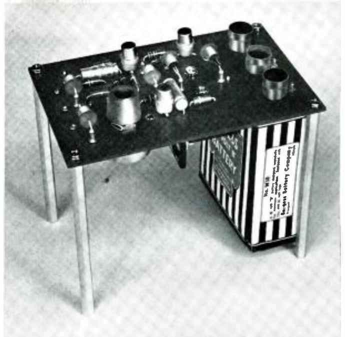
The use of an etched board permits a variety of mounting techniques. Here the unit is shown self-contained with battery.
