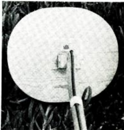
For details on the construction of the search coil, shown here, refer to text.
