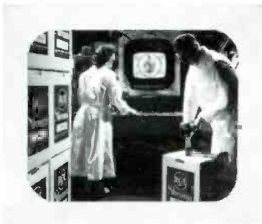
Final checkout before shipment. Here Silverama tubes receive final focus check before being shipped to customers.
