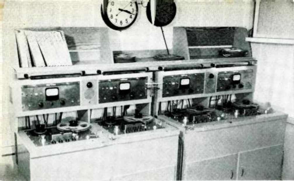
Fig. 1. The four Ampex recorders are mounted in two cabinets. These are on swivel casters and may be pulled away from the wall for access to the rear of the machines.
