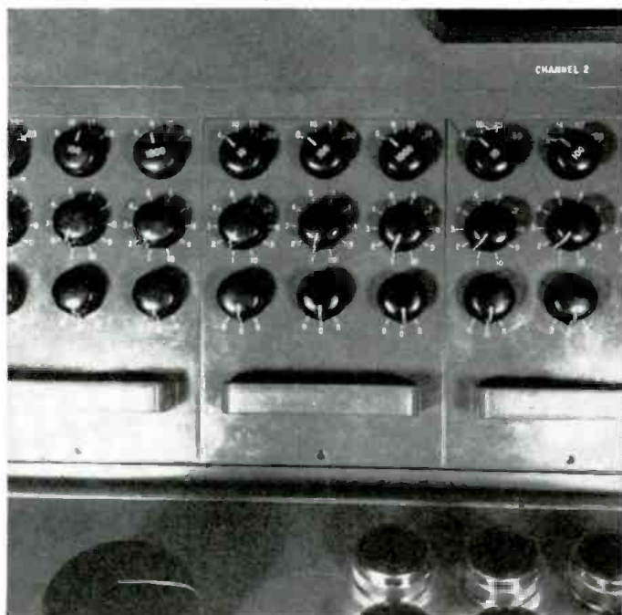
Fig. 4. The controls of the equalizing amplifier. The three knobs at the top, labeled "10," "100," and "1000," select the frequency that the operator wishes to equalize. The knob immediately below each frequency-selecting knob determines the amount of correction; the knob below that, labeled "D-O-R," selects either the "drop," "off," or "raise" characteristics.
