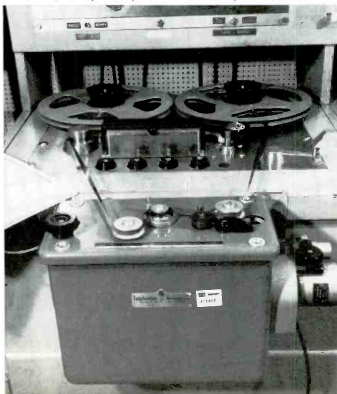
Fig. 5. The tempo regulator in use with one of the regular tape machines. The revolving head drum is the part that looks like a small pulley in a cup, in the center of the panel. The large control at the left is the speed control, and the lever knob at the right of the panel engages the capstan idler, thereby setting the tape into motion through the machine.
