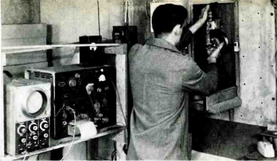
Fig. 5. Midrange tweeter is being clamped to swivel board at an anechoic chamber, in preparation for frequency-response measurements to be taken at various angles.
