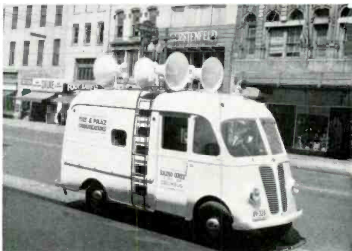
Mobile sound system using four 25-watt driver trumpets. System shown is employed for police and fire work.
