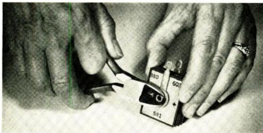
Selenium rectifier is dismantled by clipping off center eyelet.
