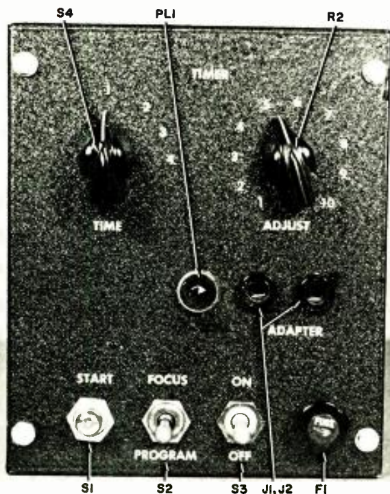
Front view showing the operating control panel of the timer.
