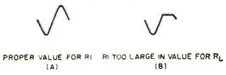
Fig. 3. Reverse biasing of the emitter-base junction cuts off the transistor and produces this clipping of the signal.
