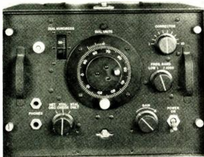
Fig. 1. Control panel of a BC-221-O. Identification plate has been removed to show crystal-oscillator padder at bottom center.
