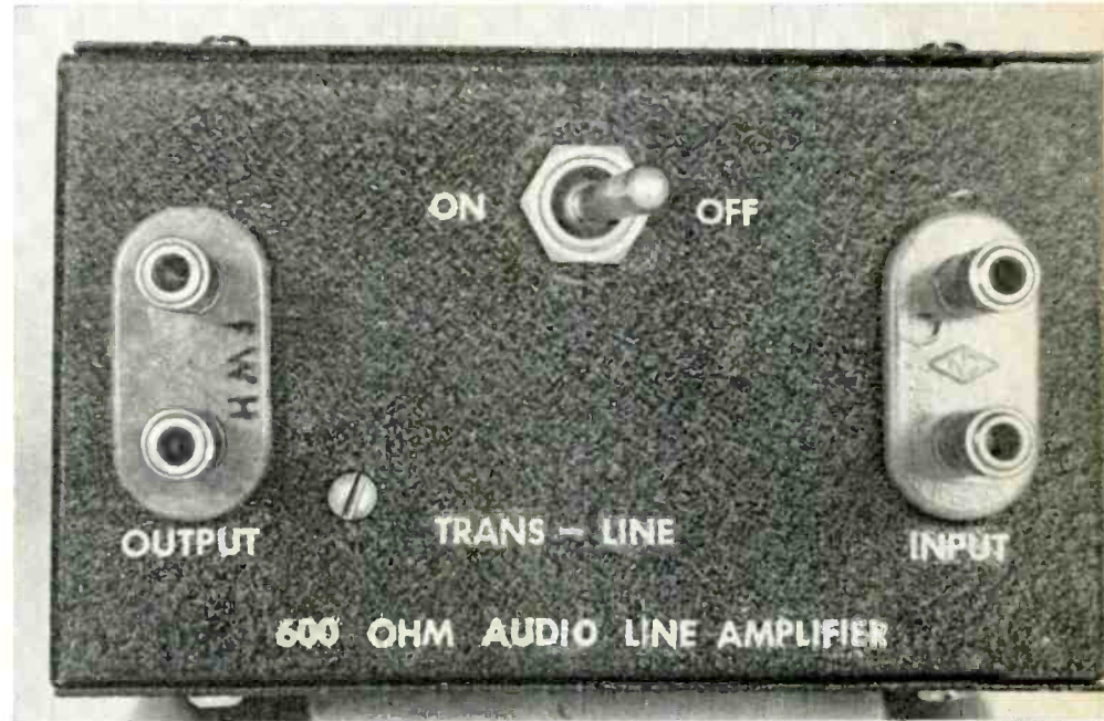
Front-panel view of the 600-ohm line amplifier, dubbed "Trans-Line" by author.
