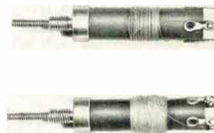
If the instructions in Fig. 2 are followed carefully, the coils will look like this. Top view shows just single-layer inside winding of T_1 . Completed coil is below.
