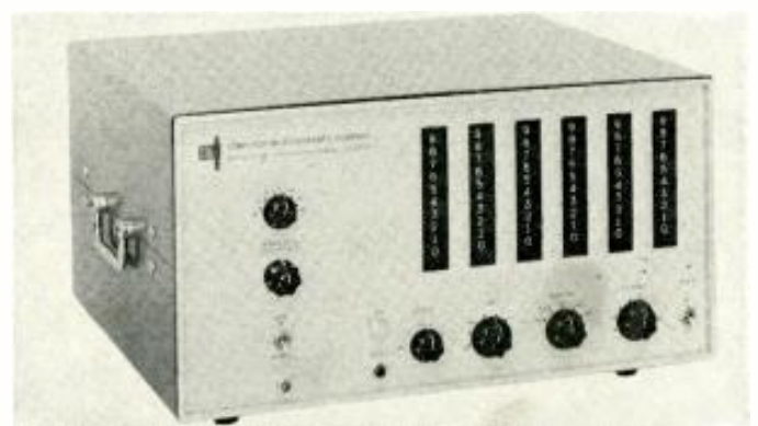
This Computer-Measurements Co. instrument is used for pulse-counting, frequency measurement. Six-decade read-out is used.
