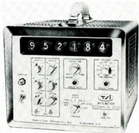
One-megacycle counter-timer made by Transistor Specialties is completely transistorized and features 6-digit in-line "Nixie" read-out.
