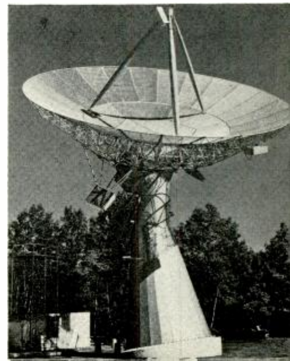
Harvard University's 60-foot parabolic dish with maser installed at feed point.
