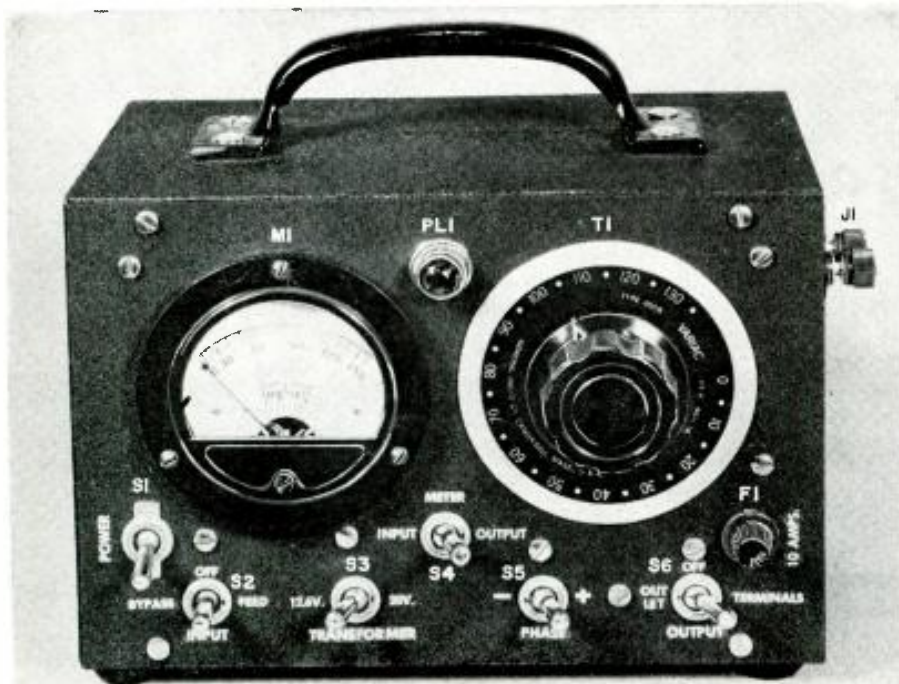
Fig. 1. Panel view of the line-voltage control box, as constructed by the author. Superimposed numbers for switches and other components correspond with Fig. 4.
