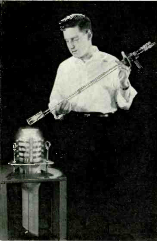
Dr. R. H. Kingston prepares the maser for the Venus observations at M.I.T. Lincoln Laboratory's Millstone Hill Radar Observatory.
