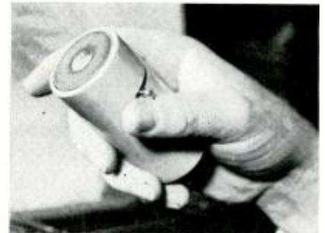
In use, the hand-held artificial larynx is pressed against the throat while the lips, mouth, and tongue are used normally. The thumb-operated control varies the pitch.
