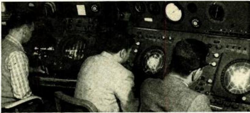
Traffic controllers at GCA radar scopes. Scopes at right are for the Airport Surveillance Radar (ASR), while those at left are for the Precision Approach Radar (PAR).
