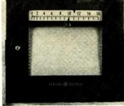
Fig. 7. This General Electric continuous recorder charts pH level changes.
