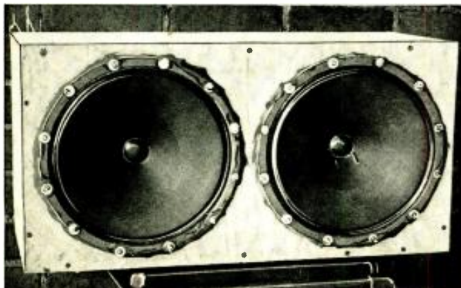
Fig. 1. Completed woofer section before covering. Speakers are mounted from front with sealing compound and machine screws.
