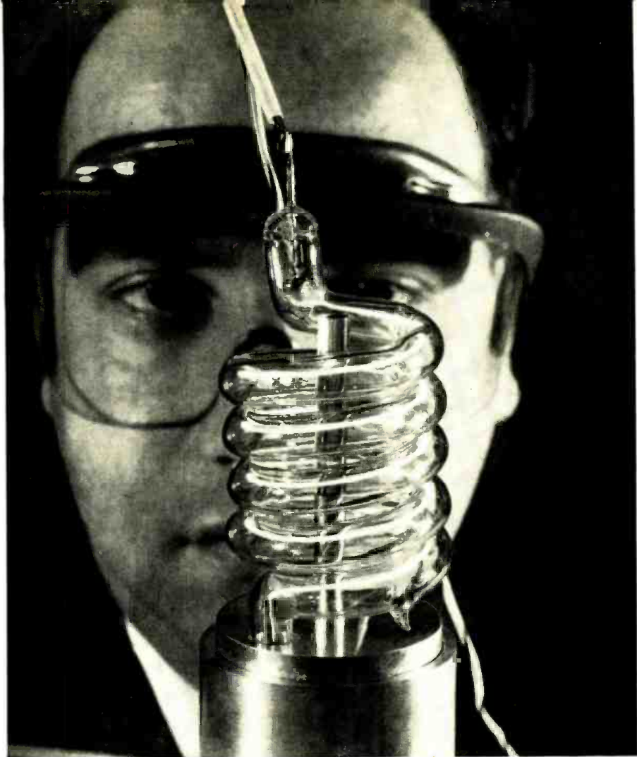
Dr. Theodore H. Maiman of Hughes Research Laboratories studies the laser's main parts. These include a light source (a special photoflash-like spiral tube) which surrounds synthetic ruby crystal rod through which excited atoms are stimulated to produce an intense beam of coherent, single-frequency light.
