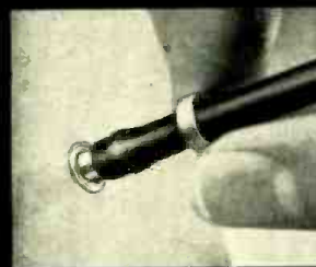
Insert the cable into the coax connector
