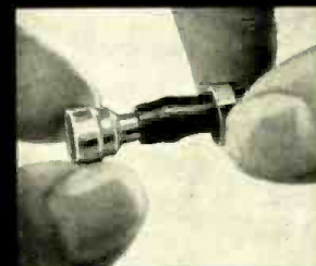
Slide the ring over the cable and insert cable into the "Q-D" connector
