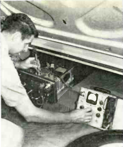
Portable test instruments are desirable, as they permit routine checking without removing units from vehicles.
