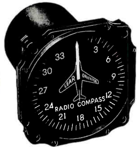
Direction indicator employed with ADF. ▶
