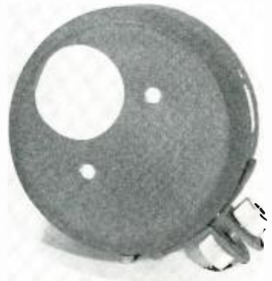
One side of the mounting board in flash-head assembly with parts in place. It fastens to the back cover with two machine screws threaded into the spacer posts.
