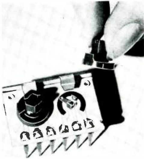
Fig. 10. Knob removed from one miniature variable resistor shows detail.
