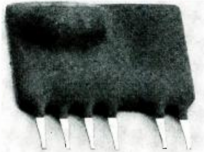
Fig. 12. Photo of phase detector package of Fig. 11. Bulge is C_5 , conventional capacitor encapsulated in unit.
