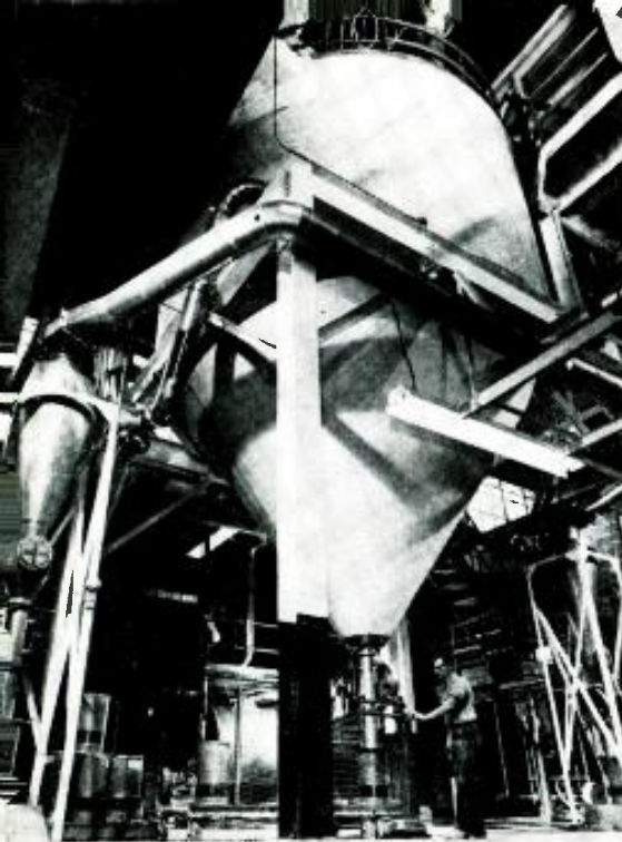
Fig. 1. Spray-drying tank for ceramic powder. Test lab is on top of tower.
