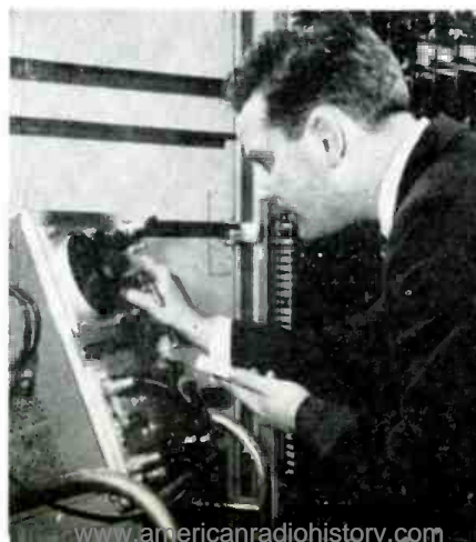
This field engineer is making a waveform check of a Univac II by Remington Rand. Rear of the Univac is in the background.
