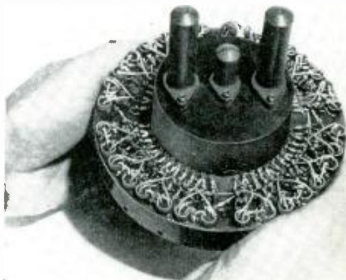
Fig. 11. Radiation sensory unit in "Pioneer III" consists of 2 large G-M tubes and small voltage supply tube.
