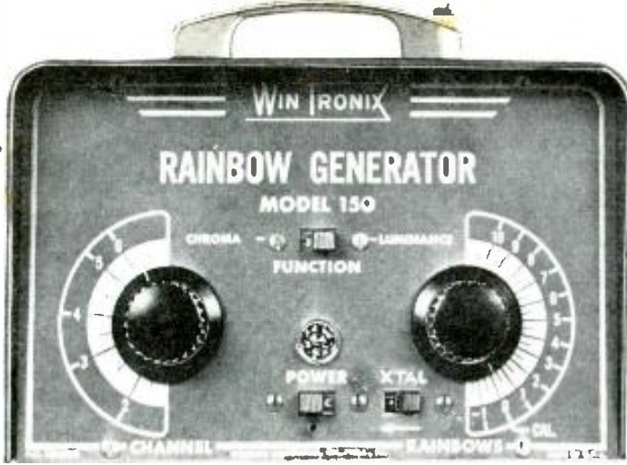
► Fig. 1. The author's altered unit, showing added switch.
