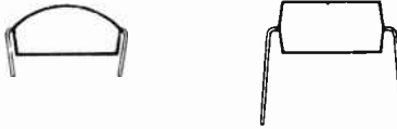
To fit inside the small pen barrel, each IC has the top ground down to a round shape and the pins cut back, as shown.
