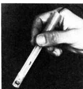
Store the pH electrode with its tip soaking in distilled water, use the protective shield and rinse with distilled water between measurements.
