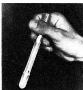
Store the pH electrode with its tip soaking in distilled water, use the protective shield and rinse with distilled water between measurements.
