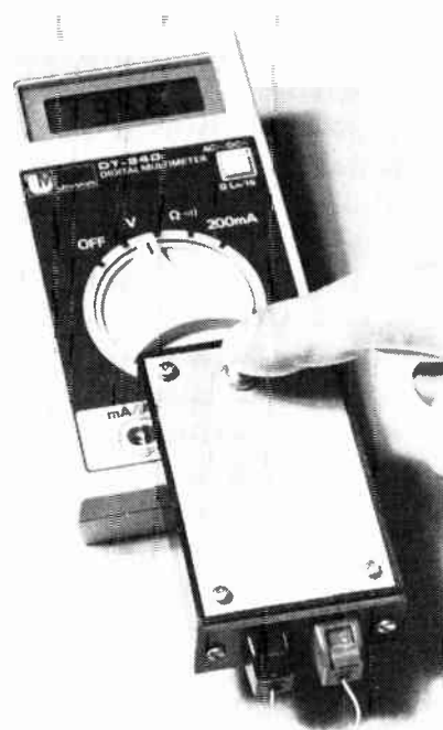
Push-to-read. The tester is housed in a 'zippy' box with banana plugs protruding from the rear spaced to suit the multimeter input sockets spacing.
