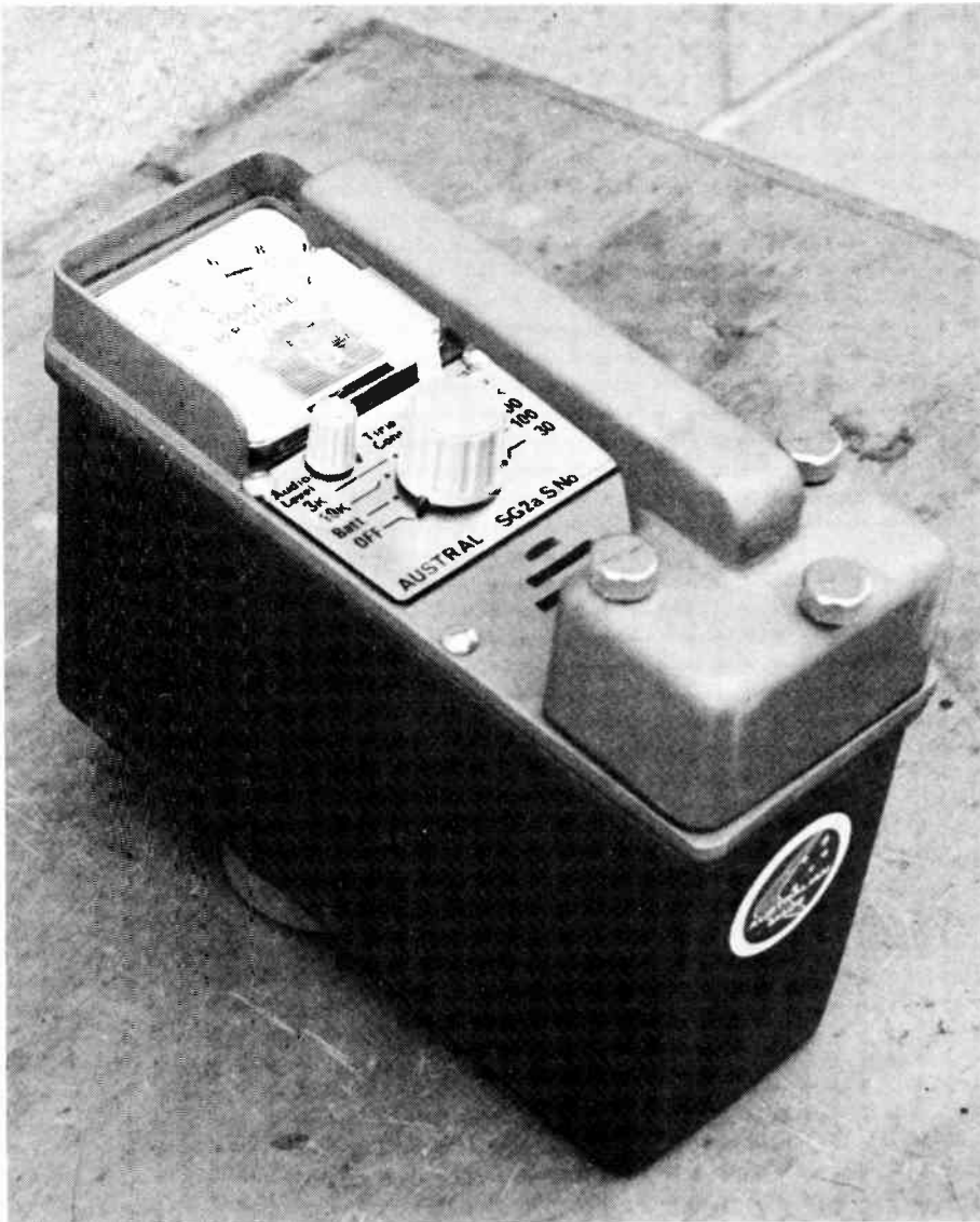
A typical scintillation counter manufactured and marketed in Australia. This model has selectable ranges and an audio output as well as a meter indicating counts per second.
