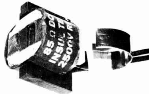
Figure 3. The search coil may be constructed from an iron-cored coil having an inductance of 1.5 Henry and dc resistance of 85 ohms.
