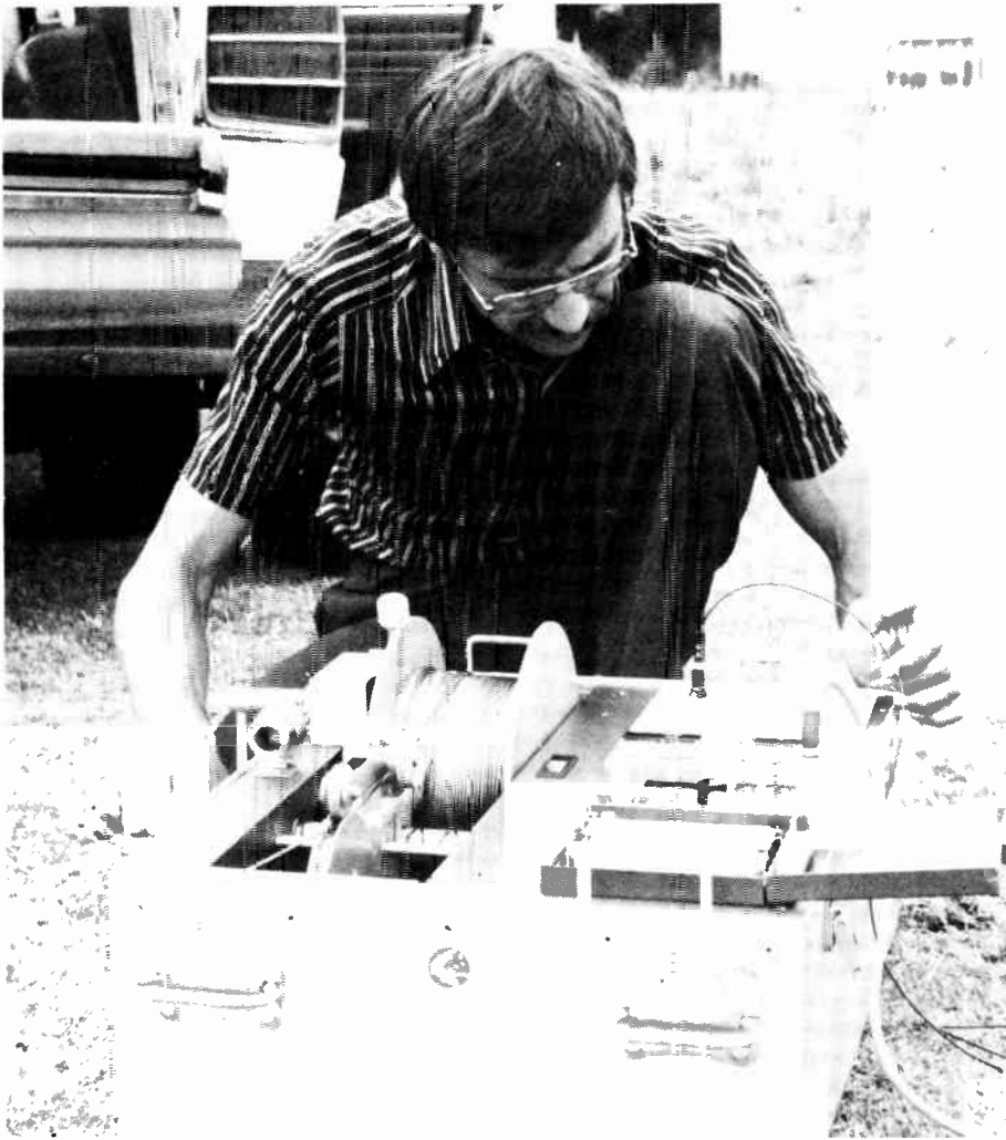
A portable radiometric borehole logger. The logging cable, which conducts power to the head and signals back, is wound off the drum at the rear of the instrument.
