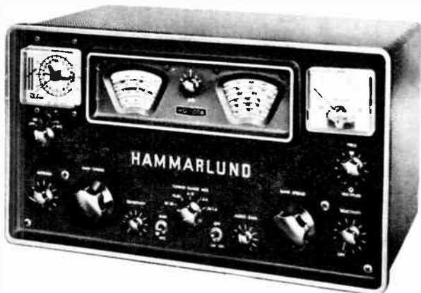
Hammarlund HQ-100A is a five-band receiver with two tuning dials; one for coarse adjustment, the other for spreading the readings. Meter at right indicates signal strengths; clock at left reads international time on 24-hour face.
