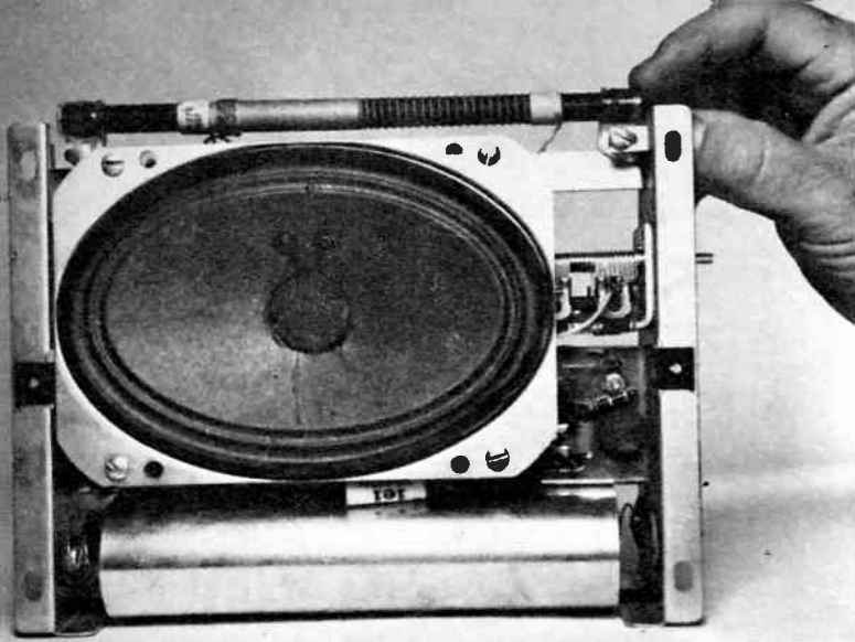
Removed from the carrying case, the chassis reveals 4x6" oval shape loud speaker, which provides excellent quality of sound. Loopstick is at top, battery compartment at bottom. Tuning capacitor is in cutout at the right of speaker.
