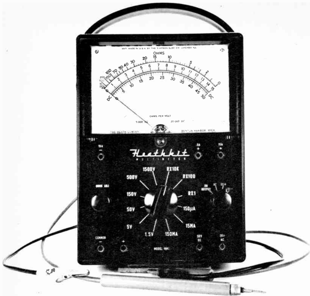
Heathkit Model MM-1 "VOM" is representative meter, easily assembled and easy to use. It measures resistance to 20 megohms, voltage to 1500, AC or DC, and current to 15 amperes. Flexible test leads plug in.
