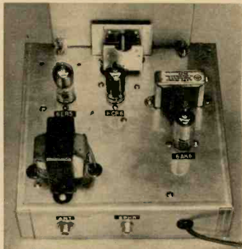
Rear view of receiver. V1 is at top, left. V2 is in center. V3 is at right below T2. T1 is at lower left. Note tuning capacitor's mounting bracket.
