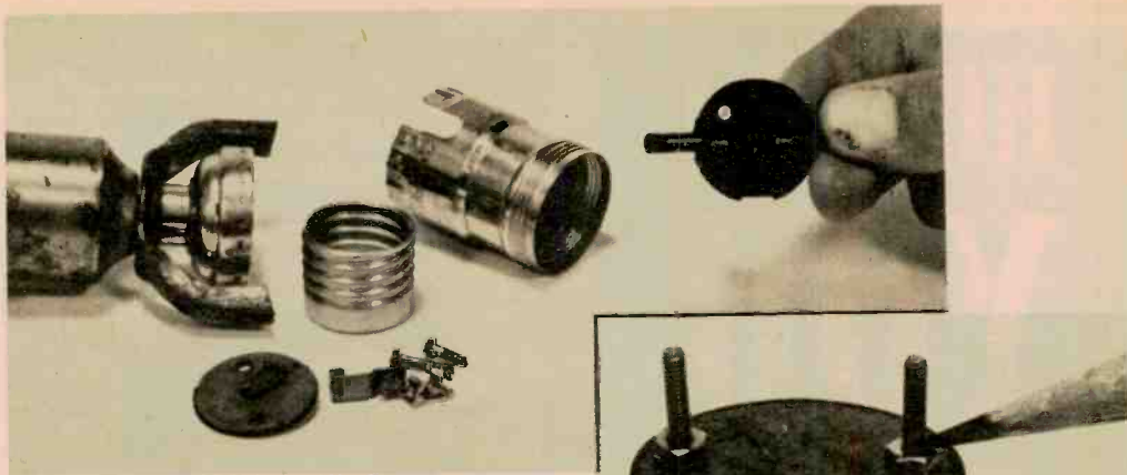
Fig. 3—If rivets were used to hold the socket together, drill them out. Discard switch assembly (in hand) but save all other parts. Cut short the screw (No. 2 or No. 3, ½ in. long) indicated by pencil—the one opposite the center-contact slot.
