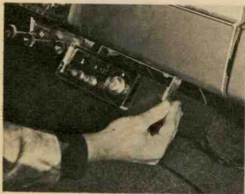
Secure transceiver with two gimbal-bracket screws, connect power cord to any hot wire under dash, attach antenna cable and the rig is ready to go.
