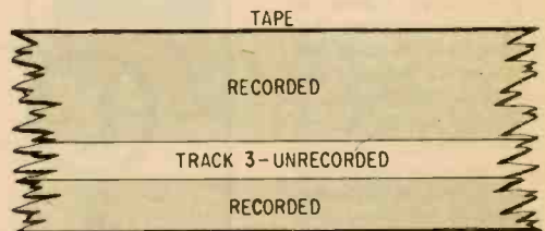
Fig. 6—Test tape will aid you in adjusting head height. You move the head slightly up or down until the output from the blank track (3) is at minimum.
