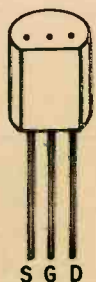
Fig. 3—Schematic of dipper. Oscillator is Colpitts. RF is detected in Q1's gate-source circuit. DC signal through gate-leak resistor R1 is coupled via sensitivity control R2 to meter M1. Use the sketch of Q1 (flat side facing you) to identify each of the leads.
