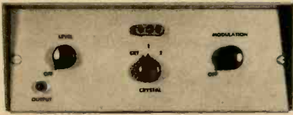
Fig. 4—Controls from left to right are output level, crystal selector, modulation level. Larger cabinet permits more front-panel crystal sockets.
