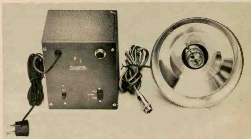
Fig. 1—Strobe consists of 4 x 5 x 6-in. power pack and 6 \frac{3}{4} -in.-dia. flash head. Flash head plugs in socket at top of power pack. Socket below is for sync cable to camera.
