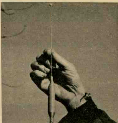
A slight adjustment in the length of the antenna section on top of the loading coil might be required to minimize the antenna system's SWR.
