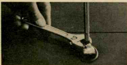
Tighten the lock nut on antenna mount with open-end wrench. Do not use pliers. Combination CB/AM antenna is ready to go since it is factory tuned.
