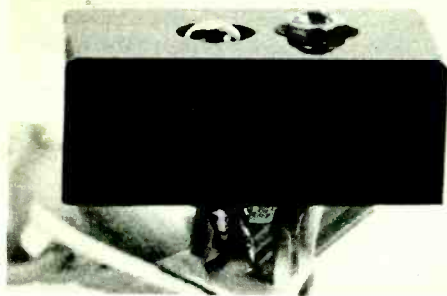
Fig. 4—Photo of plastic block, above. Note how lens of Q1 just clears top surface. Dimensions of block at right. Block material is black opaque plastic. Base lead of Q1 is cut off at case.
