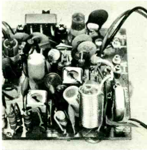
Fig. 6—Order Channel 9 receive crystal, at lower right edge of board, since walkie-talkie may not come with one. To order, see our Parts List.
