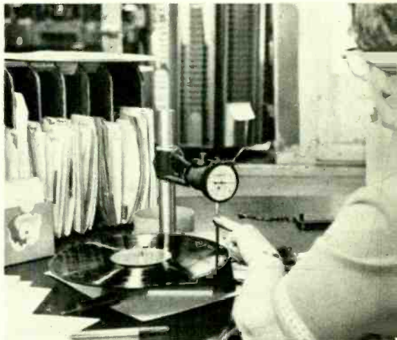
Because record's center of gravity is critical for proper operation of changer, RCA tests its Dynaflex discs for thickness at several different points.
