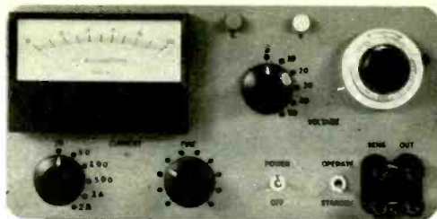
Fig. 9—Front panel indicating how various controls are labeled. Note jumpers connecting Sensing to Output binding posts—both are solid wire.
