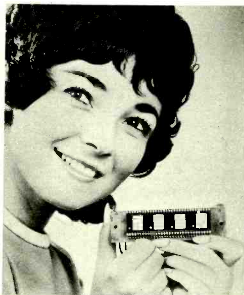
RCA's TA8040-8043 liquid-crystal readouts have four 7-segment digits, will operate from 15 VAC at frequency of 60 cps. Readouts cost $75 each.
