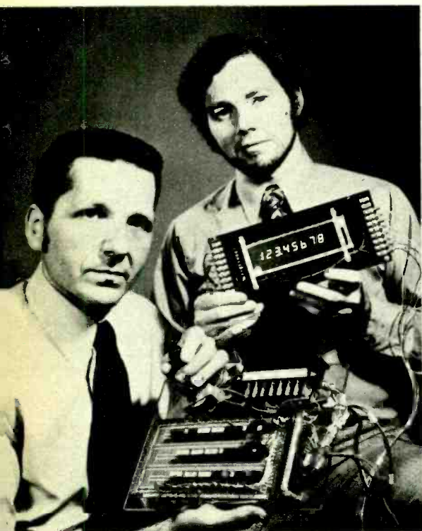
Liquid-crystal display developed by Research and Development Center at General Electric uses low- and high-frequency pulses to activate segments of 8-character readout. Circuitry is reduced 75%.
