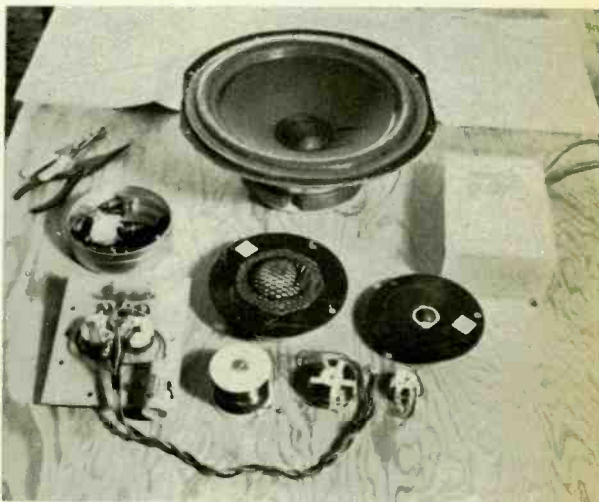
Low-frequency driver is at top; midrange and high-frequency drivers, crossover inductors are below. At the top right is 50/150 \mu f crossover capacitor.
