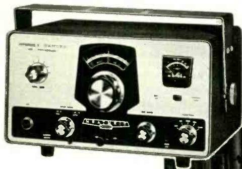
Fig. 2—The photo above shows the original Heathkit HW-32A SSB transceiver that was used for both voyages. Richard Ehrhorn, in photo at right, redesigned the rig to simplify operation and make it resistant to water damage and shock.
