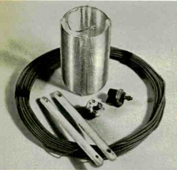
Fig. 1—Finished trap circuit, ready to be tuned to 7 mc with grid-dip meter.
