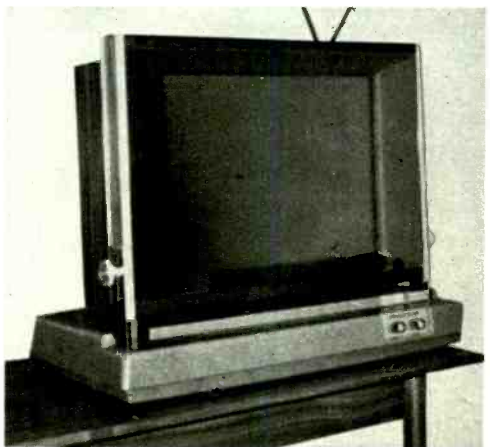
Head-on view shows mask in front of b&w picture tube. Two small knobs at lower right control color and hue—just as in a regular color TV.
