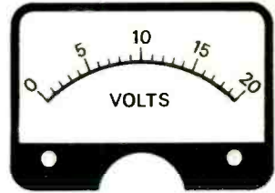
Fig. 4—Scale shown is for 17-V model. Draw new meter scale and double numbers for 38-V supply.
