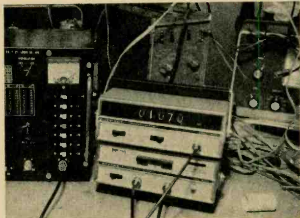
Fig. 12—Heathkit IB-102 scaler (under counter) can divide up to 150-mc signal by 100 or 10. 107-mc readout is of FM generator.
