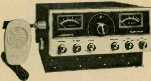
23RD PRIZE: Lafayette Radio's Telstat SSB-25 one of the first CB rigs with SSB on all 23 channels. This results in 46 operating channels and 15 watts PEP input power.
