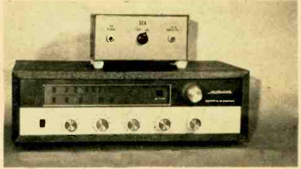
Fig. 2—SCA adaptor ready to be connected to FM tuner. Tuner must have wide-band ratio detector or discriminator that handles stereo-FM broadcasts.
