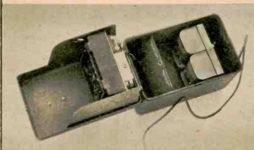
Fig. 1—Heathkit circuit board (left). Case (below) holds batteries and stores transducer. Right photo shows our method of mounting transducer on end of 4-ft. pole that can be lowered into water.
