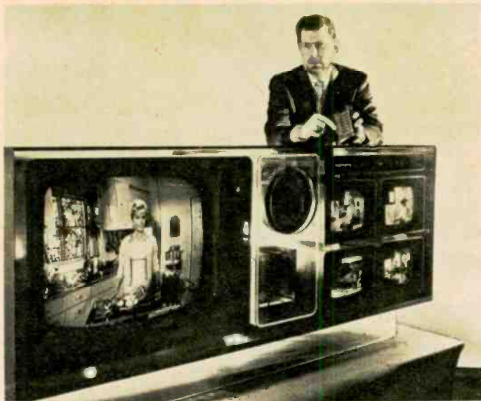
Five in one. RCA now is showing a $250,000 prototype of a color TV that has five screens. The futuristic Showcase '70 has provisions for simultaneous viewing of five different programs and a remote control that will switch the program on one of the small monitors to the large center screen.
