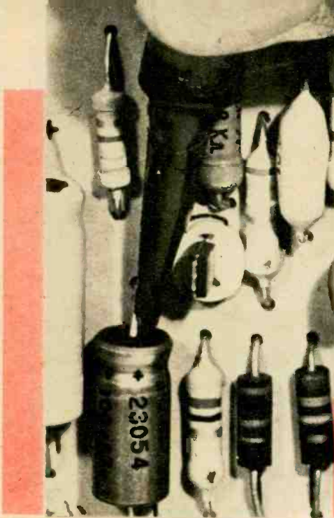
Fig. 3—Note crowding in left photo. To avoid shorts, which will destroy transistors, cover end of test probe down to tip with tape. Large electrolytics (above) have big charge that should be removed with 500-ohm, 1-watt resistor.
