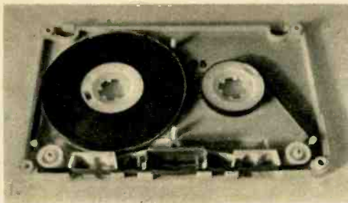
A scene which few get to see—the interior of a Philips-type cassette. The big question now is can Dolby and Crolyn make this device the new LP?
