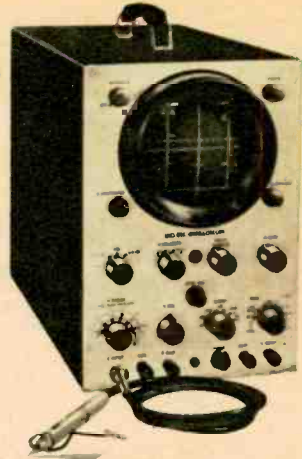
RCA Model WO-91C scope costs $269, offers choice of narrow- or wideband response. Newer version is the solid-state WO-505A.
