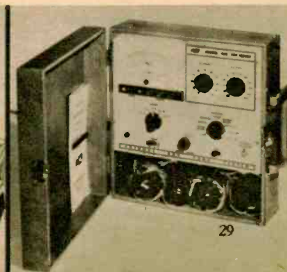
B&K Model 465 CRT tester costs $99.95, will test and rejuvenate both color and b&w CRTs in set.
