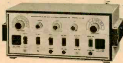
B&K Model 1245 color bar generator (above) costs $139.95, has 5000- \mu V output. Patterns are bars, horiz. and vert. lines, crosshatch and dot.
