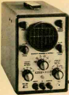
Elco Model 435 wideband DC scope costs $119.95 ($169.95 assembled); the frequency response is flat out to 4.5 mc.
