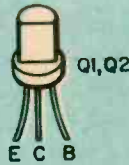
Fig. 3—Be sure of the identification of the leads of transistors Q1 and Q2. Sketch at right aids in identifying them.
