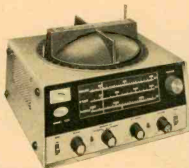
Model DF-1301 direction finder made by Sonar costs $249.50. It works on both AM and beacon stations.
