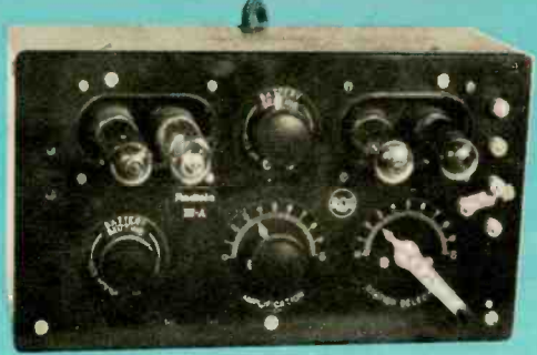
Above is Westinghouse Electric's Radiola III-A manufactured in 1924 for RCA. Circuit uses four WD-11 tubes; has regen detector, push-pull output.
