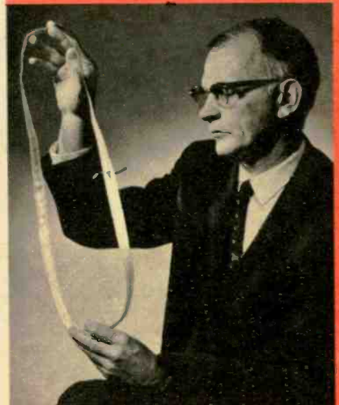
Richard L. Davis, inventor of Moebius resistor, shows how this component looks before it's bundled into a compact package.
