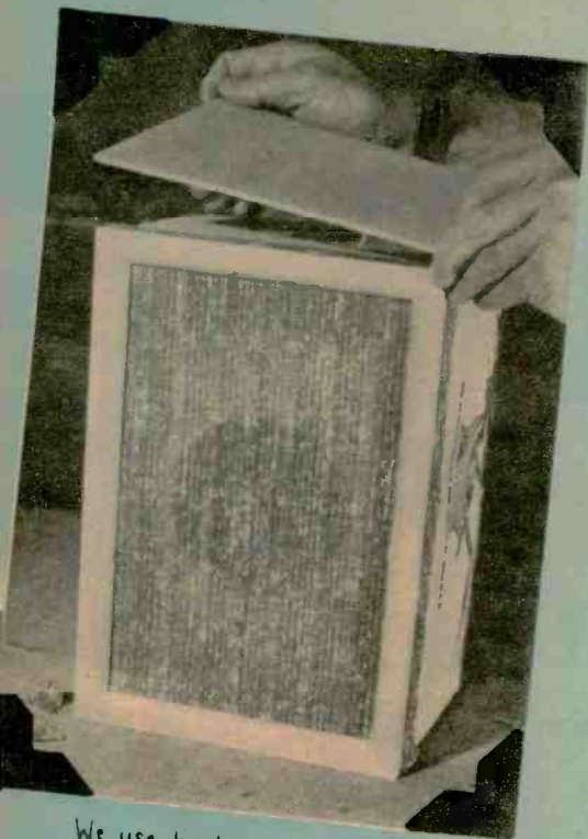
We use linoleum paste again to attach the grille cloth and frame. Eighth-inch plywood is used to dress up the outside.
