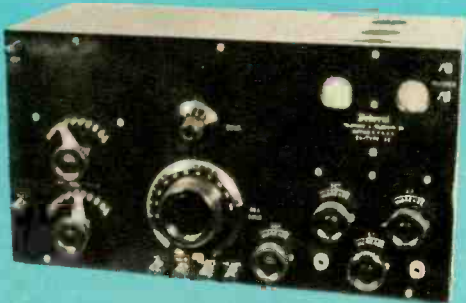
Above is Federal 58 manufactured in 1922. TRF circuit has one RF stage, two audio stages and detector. Battery-powered set uses four tubes.
