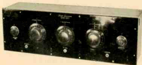
Above is Freed-Eisemann Model NR-5 manufactured in 1923. Three-stage TRF-Neutrodyne circuit uses five 201A tubes. It's also battery powered.
