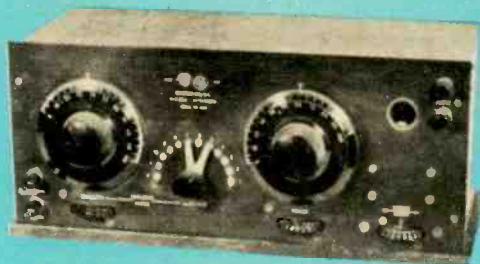
Grebe Model CR-5, above, was manufactured in 1921. Regenerative detector circuit uses one tube (either 200A or 201A) and is battery powered.
