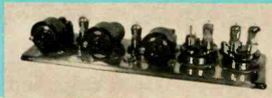
At right is Atwater Kent Model 12 manufactured in 1923. Six tubes are used in circuit having three TRF stages, a detector and three audio stages.
