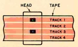
Fig. 5—To prevent crosstalk between tracks, head height must be correct. For example, if head is too low, tracks 1 and 2 will pass over upper gap.
