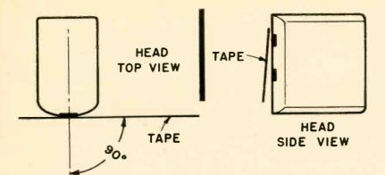
Fig. 6—Contact angle (left) is tangent at which tape contacts head. It should be 90° to head's centerline. Tilt (right) is deviation from parallel between surfaces of tape head and tape. Tape and head should be exactly parallel at contact (it's shown away from head here for illustration purposes).
