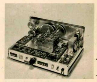
The Allied Model A-2515 receiver has four printedcircuit boards on chassis. Note the three-gang main-tuning and bandspread variable capacitors.
