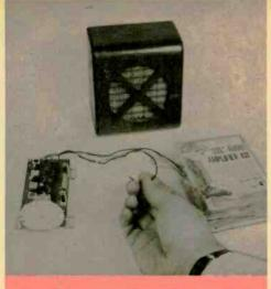
Once Science Fair OTL amplifier kit is wired, components fit back into plastic case. Here, low-level signal from AM tuner is amplified.
