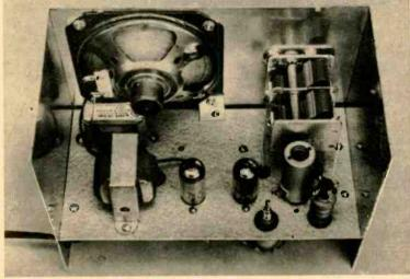
Top of chassis. Output transformer is near speaker. Mount power transformer (with core turned 90 degrees with respect to output transformer) behind it. Transformer T1 is at lower right corner of chassis.
