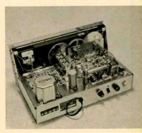
Radio Shack DX-150 has three-gang tuning capacitor and smaller bandspread capacitor to right of it. Power transformer is in lower left corner.
