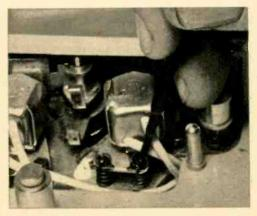
Fig. 8—On same machine azimuth-adjustment screw is at rear of head on the mounting plate. Use demagnetized tools when working around head.
