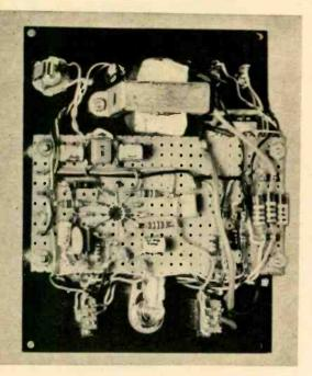
Fig. 1—Mount parts on panel with long leads, then wire board. Install board with 1-in. spacers so back of board doesn't touch panel parts.
