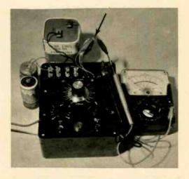
Fig. 3—Alligators hold test FET (arrow). D cells are for gate bias voltage, lantern battery supplies FET's drain voltage; VOM indicates the null.
