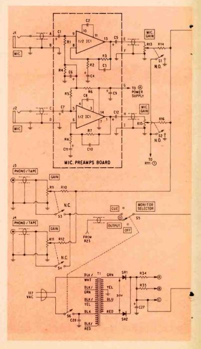
The program/VU-amp. board is assembled in the same manner except that C15 and C20 (same physical position on the board as C12, C5) must be  $6 \mu f$ .
