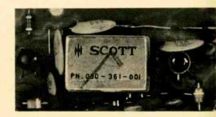
Scott model 342C 100-watt stereo FM receiver is latest component to feature quartz-crystal lattice filter. Factory alignment is said to be permanent. The check mark was put there by factory.
