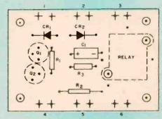
Blister packages and pegboards are trademarks of minikits. Parts placement diagram above for RCA kit is typical aid included for builder.
