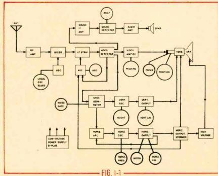
Block diagram of basic circuits found in b&w and color receivers. Signals consisting of picture information, sync. blanking pulses and FM sound are distributed at video-detector.
