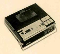
remote use. Switch allows selection of either internal mike, external mike or simultaneous use of both. Tape speeds: 1% ips, 3¾ ips, 7½ ips and 15/16 ips for extra-long playing time. \$229.50. Superscope Inc., 8150 Vineland Ave., Sun Valley, Calif. 91352.
