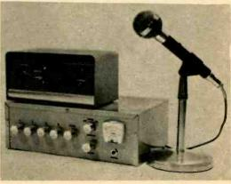
Fig. 7—Ready to go on the air. Wireless broadcaster can be near console. For best range put it in attic near antenna and feed audio up to it.
