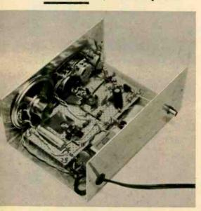
To allow room for installation of perforated board, mount power transformer against the rear of cabinet. Speaker is cemented to panel with epoxy.
