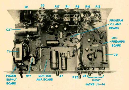
Fig. 4—Photo of inside of console shows part locations. Mount cabinet parts before installing boards.
