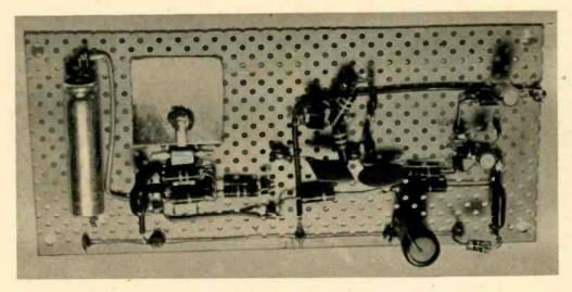
Metal tab is IC's tin heat sink. Note long leads on diodes (lower right) to prevent soldering-heat damage.
