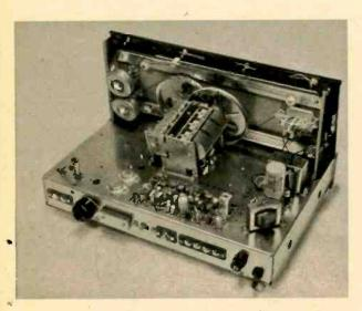
The Latayette HA-600T receiver has a good deal of circuitry packed on one printed-circuit board. Output transistors are to the left of the board.
