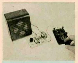
IC minikit from RCA serves as code practice oscillator. Missing items (like key and speaker) must be supplied by experimenter.
