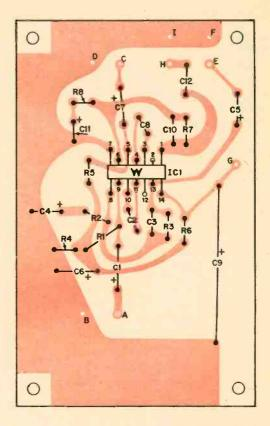
Fig. 1—Below is template for mic.-preamps and program/VU-amp. boards. Trace outline of black areas with carbon paper on foil side of two boards. Part numbers and location for mic.-preamps board is above. Fig. 8 has program/VU-amp. board nos.
