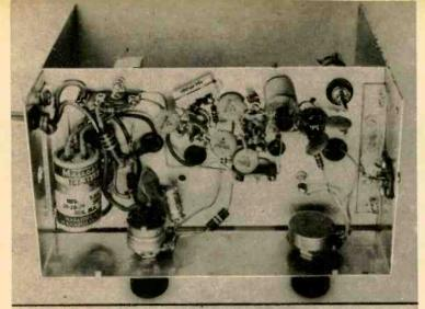
Underside of chassis. Note how the chassis in our model is held in the cabinet with angle strips. If this material is not available, use four angle brackets. Antenna jack (J1) is at right.
